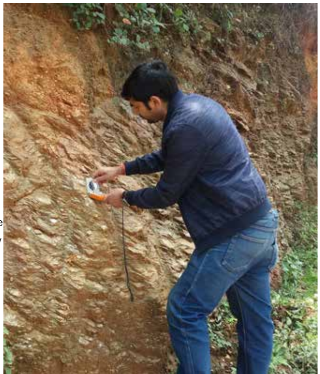
Measuring rock dip and strike direction using a clinometer
