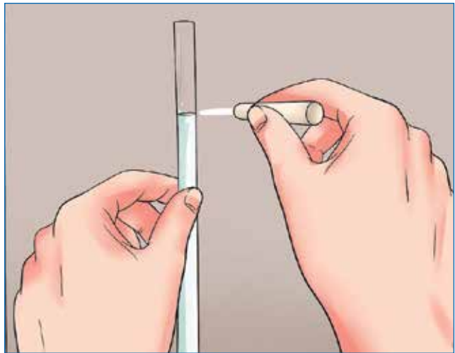
Figure 47: Marking the Level Transferred
