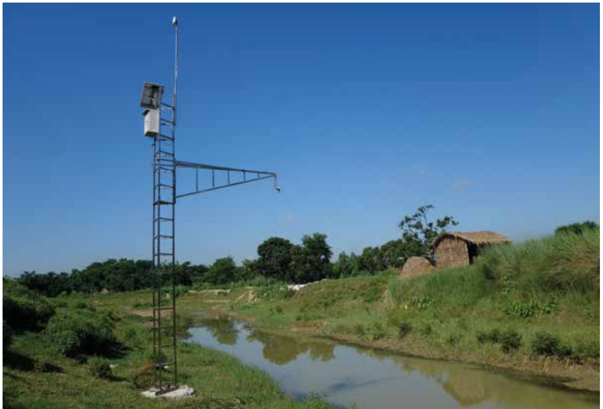
A CBFEWS data uploading unit in Bhitamora, Bihar, India
