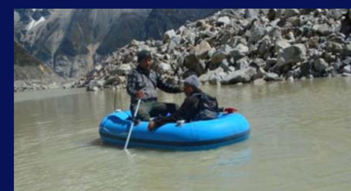
Bathymetry survey (measurement of glacial lake depth)
