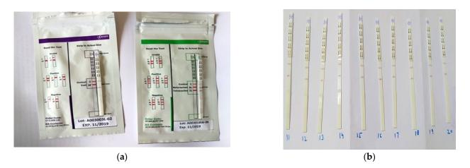
**Figure 3.** (a) Manual reading of Charm ROSA Dip Kit strip; (b) actual picture of Charm ROSA Dip test kit strips used in the test.
