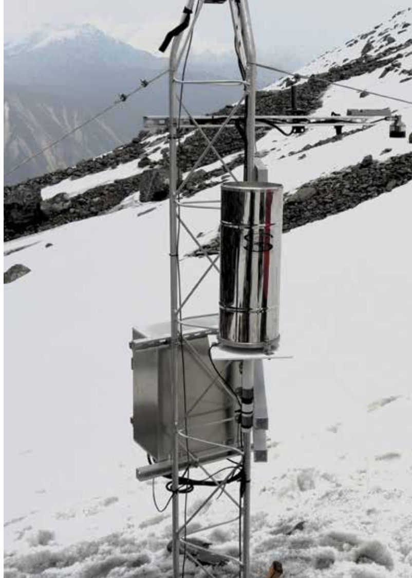
Figure 9: Tipping bucket precipitation gauge installed on the upper station
