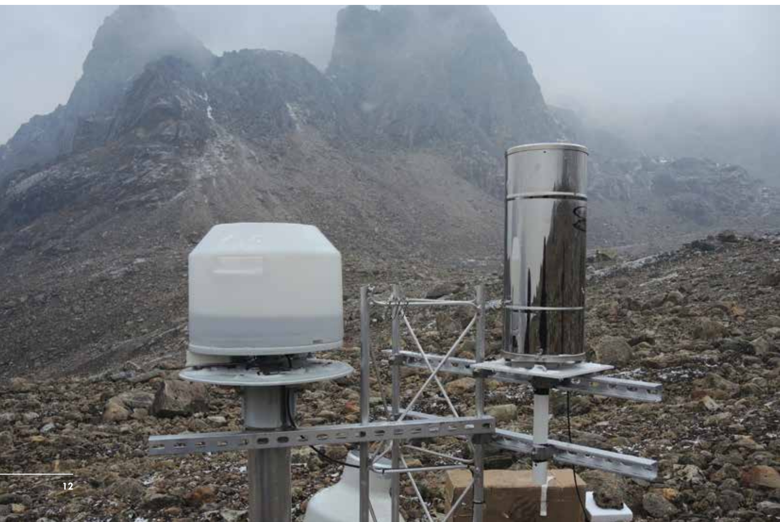
Figure 8: Secondary mast on Ganja La station, after installation of the tipping bucket
