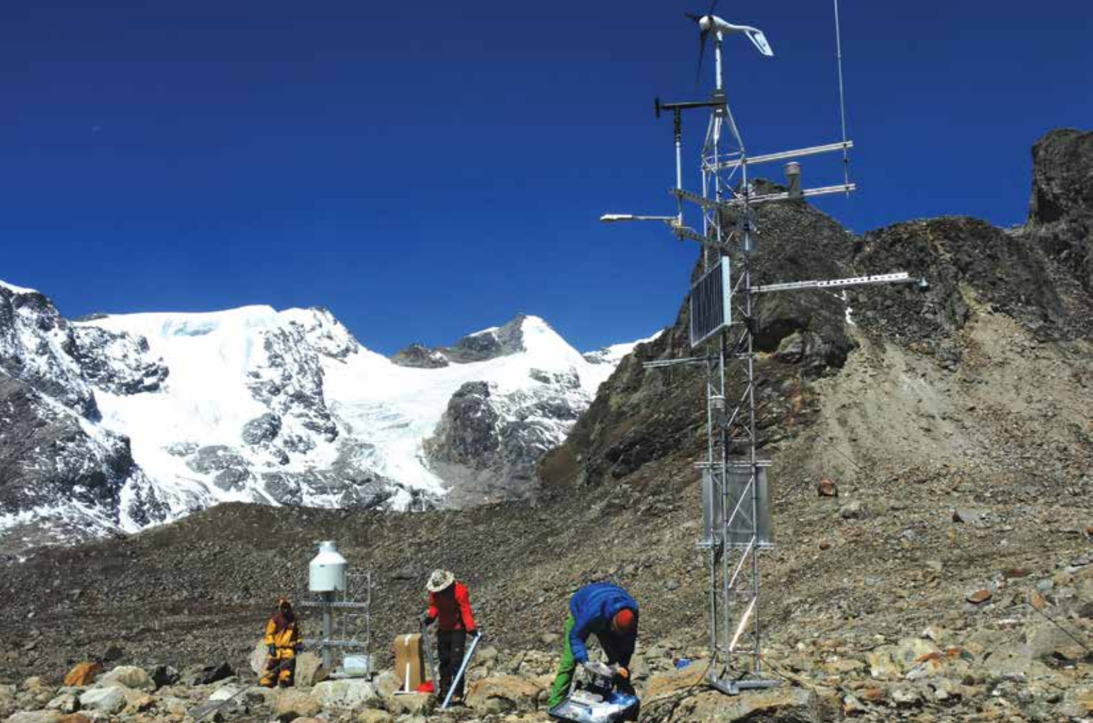
Figure 7: Installation of the tipping bucket and maintenance of the weighing gauge (Ganja La station)
