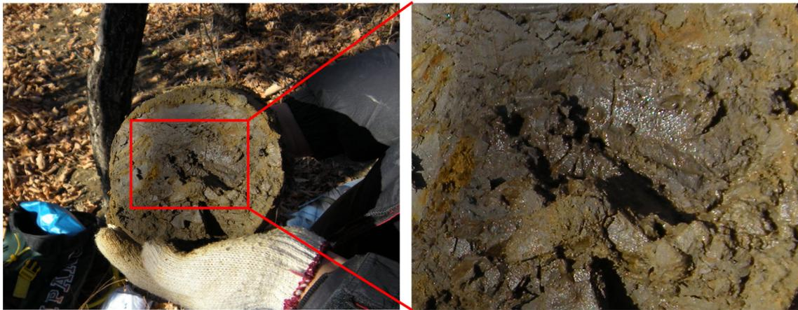
**Fig. 14** Photo of high-temperature permafrost. Sampling location is on survey line III–III', at the 40-m position on the *x*-axis. Drilling time is May 2010
