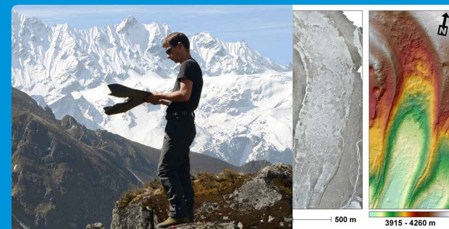
High-resolution monitoring of Himalayan glacier dynamics using unmanned aerial vehicles on the debris-covered Lirung Glacier
