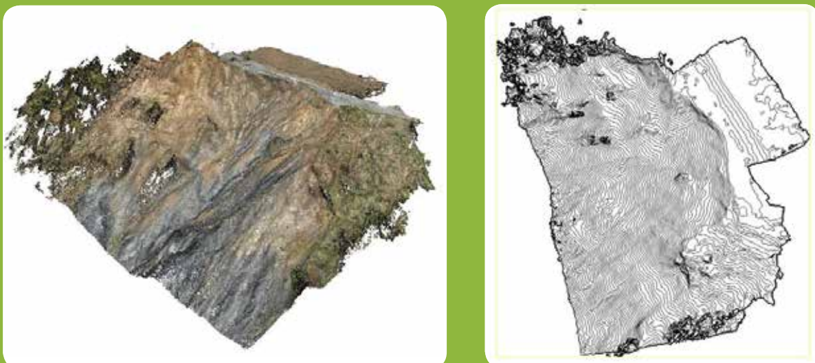
Figure 20: High resolution terrain model (DEM) using Lidar and unmanned aerial vehicle (UAV) are becoming popular tools to study surface processes, including landslides
