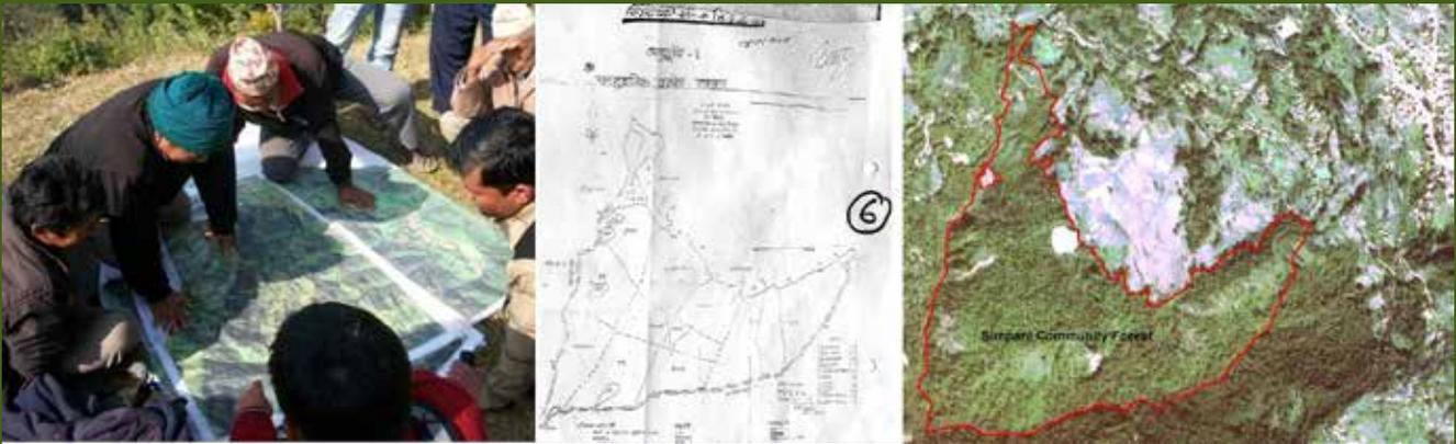
contours, settlements, roads and trails, and streams for each watershed. A 20 m digital elevation model (DEM) was generated from the contour and spot height layers using the topogrid model of ArcGIS.
