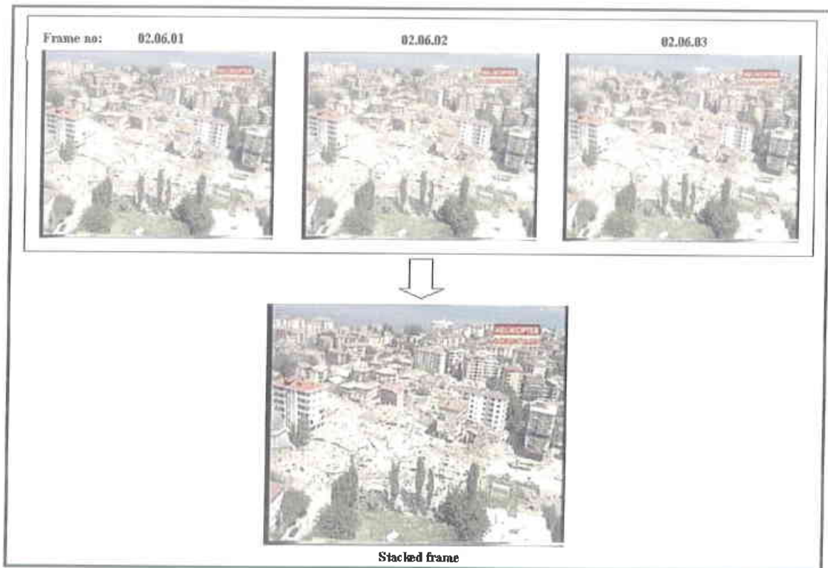
Figure 7.6. Image stacking process to enhance the video frames for further image processing
