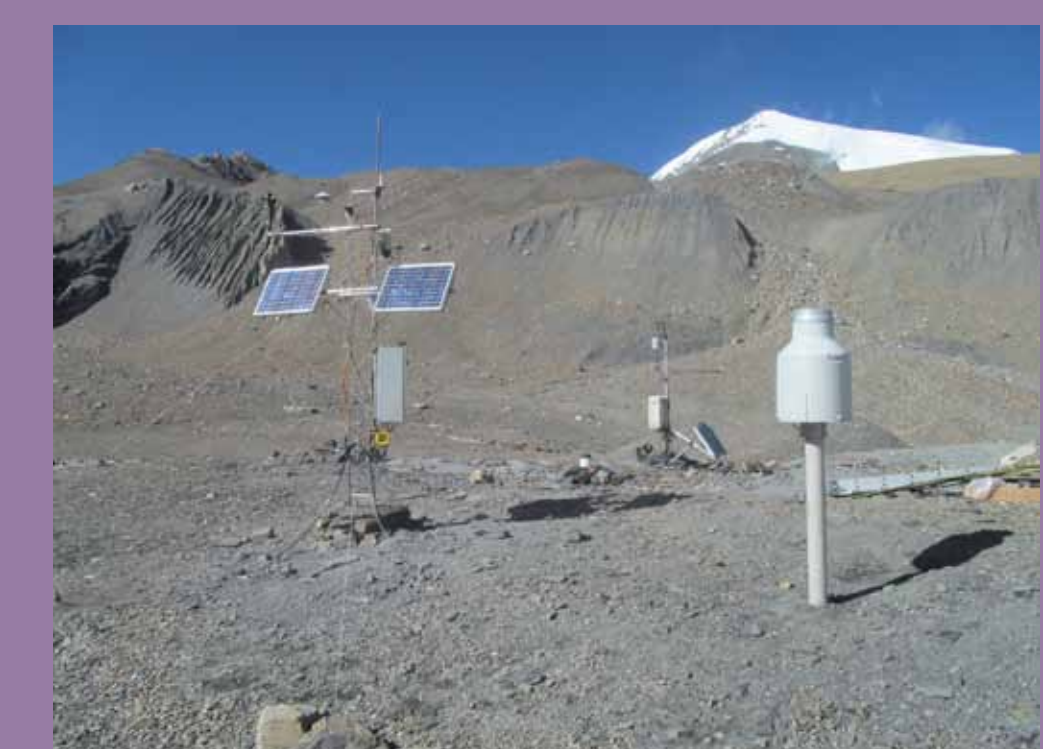
Automatic Weather Station at Rikha Samba Glacier Base Camp
