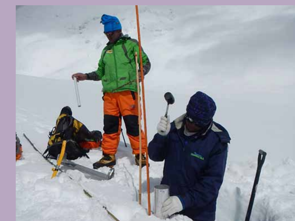
Snow density measurement on Rikha Samba Glacier
