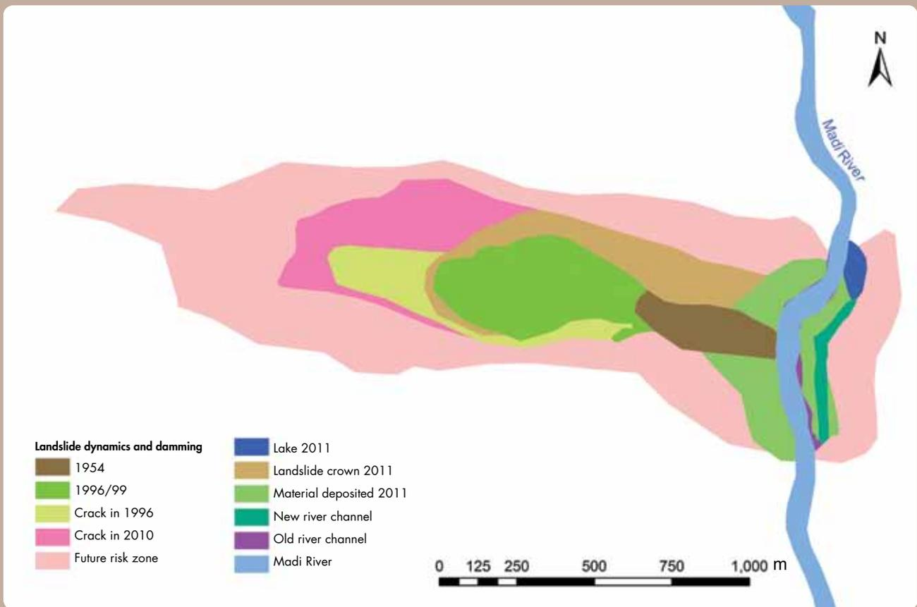
the river cut the dam and the left bank of the river generating a 5 m flood downstream, which damaged a suspension bridge at Chasu, among other things.
