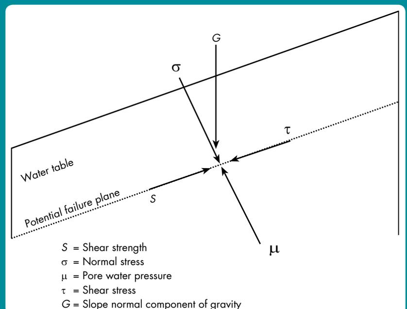
$FS > 1$  indicates stable slope conditions. According to Vazirani and Ratwani (1980) the factor of safety against sliding should be not less than 1.5.
