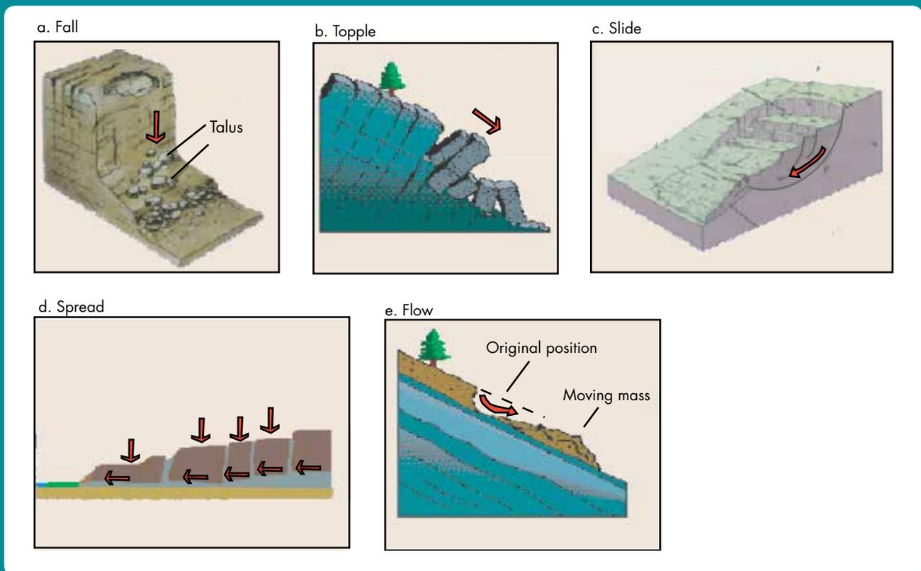
**Slide.** A slide is a down slope movement of rocks or soil occurring mainly on surfaces of rupture or relatively thin zones of intense shear strain. There are two major types of slide: rotational and translational. Rotational slides occur most frequently on the surface of homogeneous slopes, whereas translational slides take place on more or less plane surfaces.
