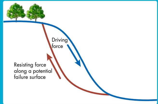
Figure 3: Force diagram for thin to thick translational slides
