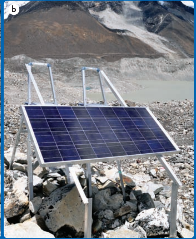
Figure 6: Monitoring of Imja glacial lake: a) field server the lake (2009); b) solar panel for field server (2009); c) part of image from field server at lake (26 June 2009); d) part of image from field server at Namche Bazar (1 Jan 2010)
