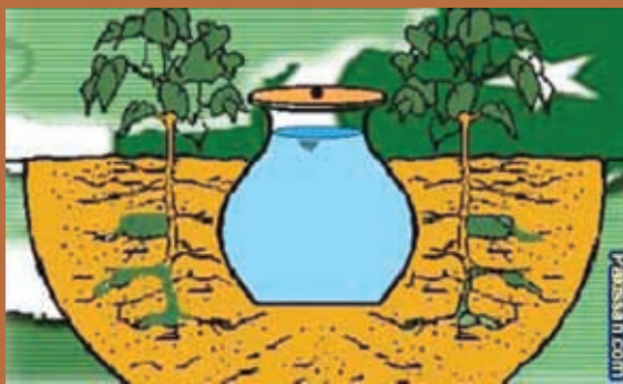
Figure 4: Pitcher irrigation and pitcher filled with water.
