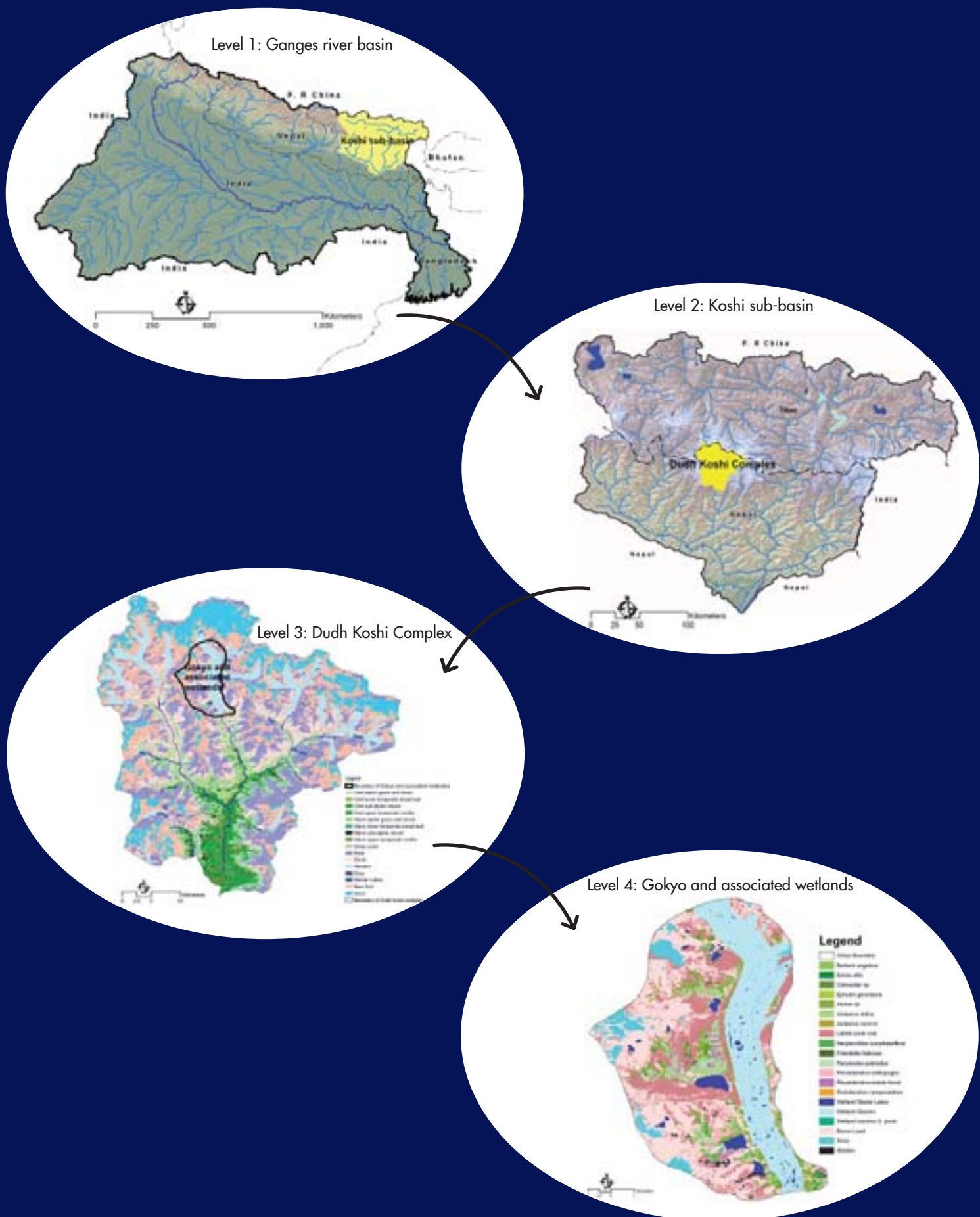
Figure 2: The four-tiered landscape (multi-scale) approach for wetland inventory. The level of detail varies with spatial scale in the four-level hierarchy from river basin to wetland habitat
