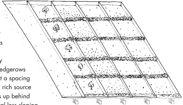
A series of plots were established in 1995 to measure the impact of nitrogen-fixing hedgerows on soil erosion and investigate the conditions that favour or hinder erosion. The surface runoff from each experimental plot is diverted through a gutter system into collection tanks and the soil erosion is evaluated from sediment concentration in runoff and total runoff.
