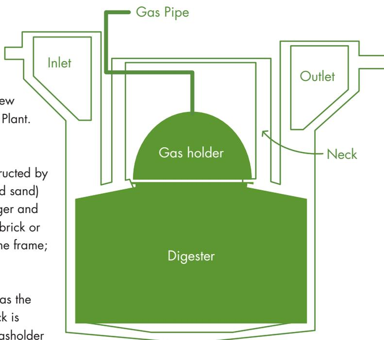
**Gasholder:** The gasholder is made of reinforced glassfibre which is 100% air and water tight. The diameter of the gas holder is 1.6 m; the volume varies with the height.
