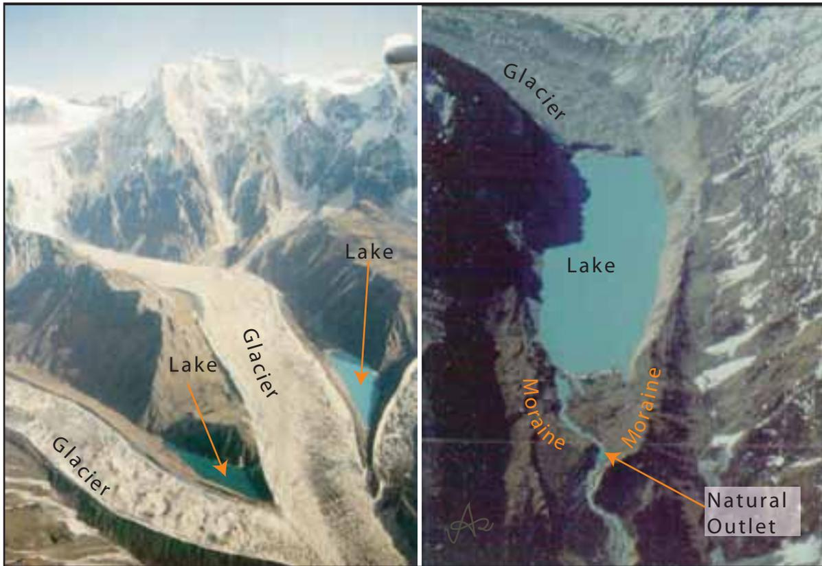
Figure 19: Typical ice-dammed (left) and moraine-dammed (right) lakes
