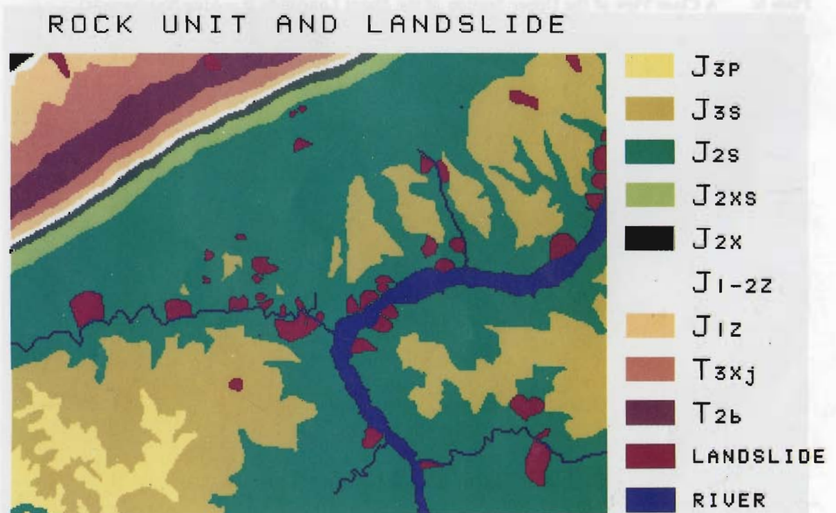
J 3p Ponglaizhen Group, J 3s Sulning Group, J 2s Shamiaogi Group A, J 2x Xintangou Group, J 1-1-2z Zilioujin Group, J 1z Zhengzhuchong Group, T 3xj Xujiuhe Group, T 2b Badong Group.
