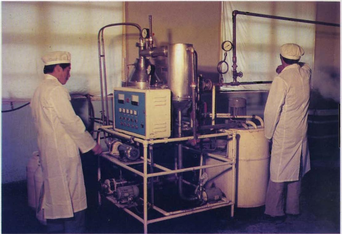
Seabuckthorn raw juice has to be condensed to transport it to the terminal processing factories. In this picture, the workers of Xiaojin Seabuckthorn Beverage Factory, Western Sichuan, China, are operating the condensing machine.
