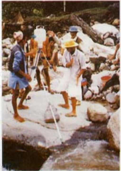
Figure 17: Preparation for a tracer measurement with a Mariott Bottle at the main hydrological station, Yarsha Khola Watershed, Nepal (photo: monsoon season 1997)
