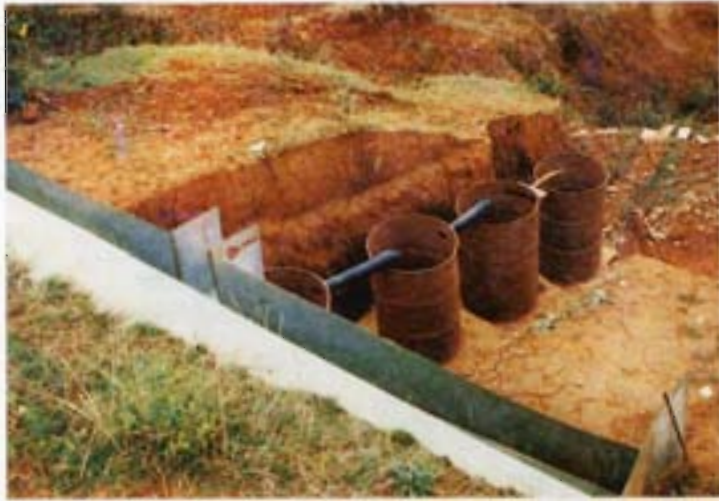
Figure 22: The gutter and the collection drums of an erosion plot in Namdu, Yarsha Khola Watershed, Nepal (photo: May 1998)
