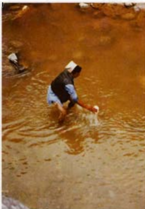
Figure 19: The reader taking a sample of suspended sediment at the main hydrological station in Yarsha Khola Watershed, Nepal (photo: monsoon season 1997)
