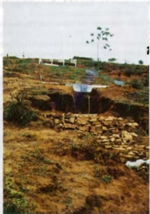
Figure 6: The erosion plot on red soil in Namdu, Yarsha Khola Watershed, Nepal (photo: May 1997)
