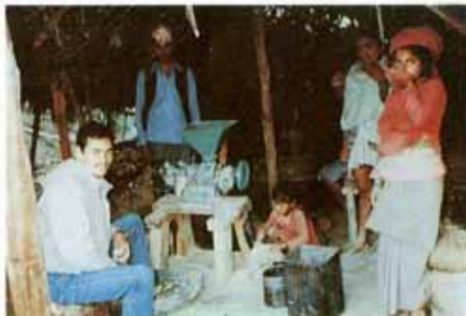
Paddy De-husker Operated by Micro-hydropower Plant Multipurpose Power Unit at Gajuri, Dhading District, Nepal
