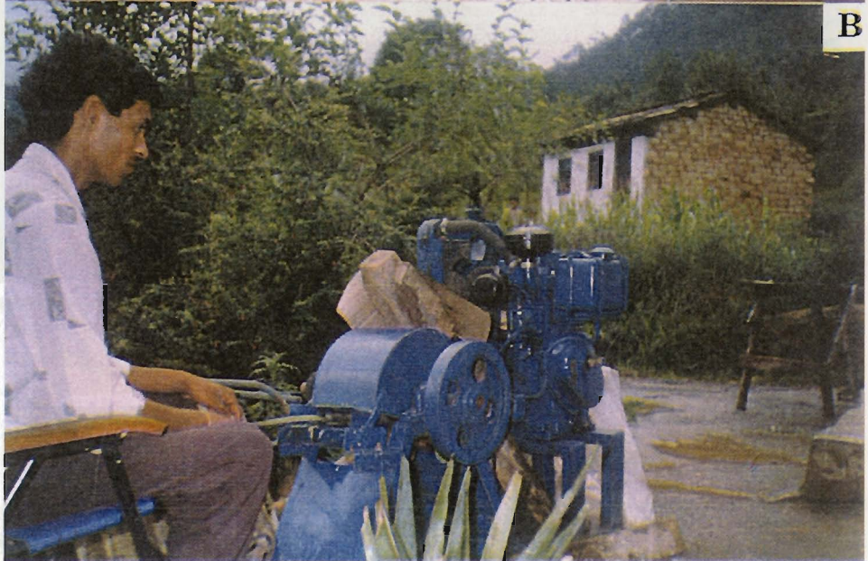
Plate 4.4: Development of Technology A) Primitive, manual method of scutching Agave fibre B) Modern machine developed for the extraction of fibre
