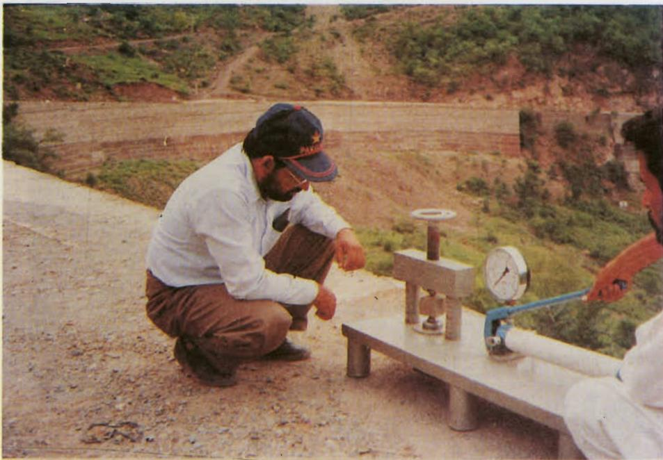
Plate 16: Point load testing of rock at site
