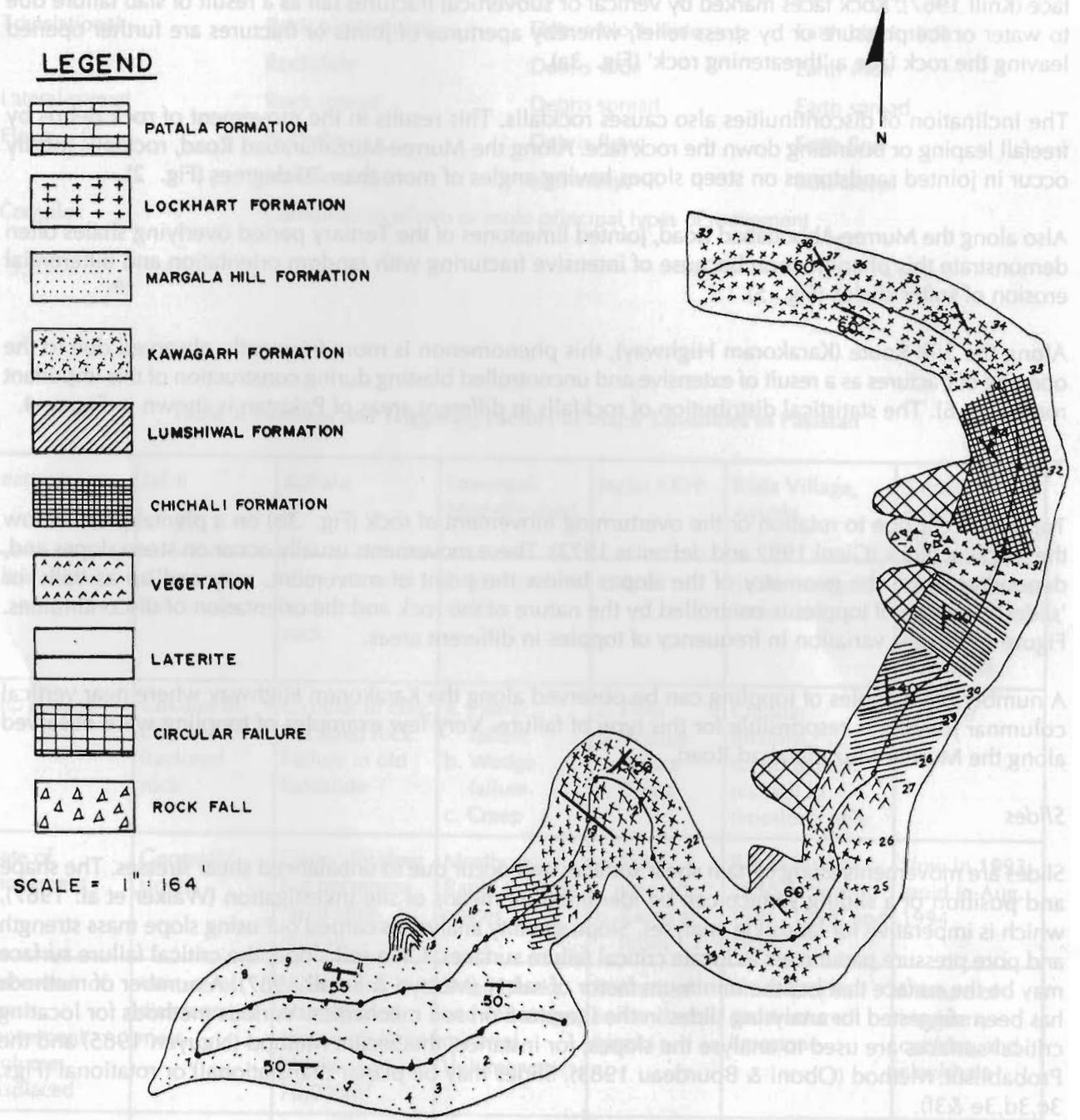
Figure 6: Stability Assessment along part of the Karakoram Highway from Thakot to Batgram (28km) Using the Stereoplotting Technique
