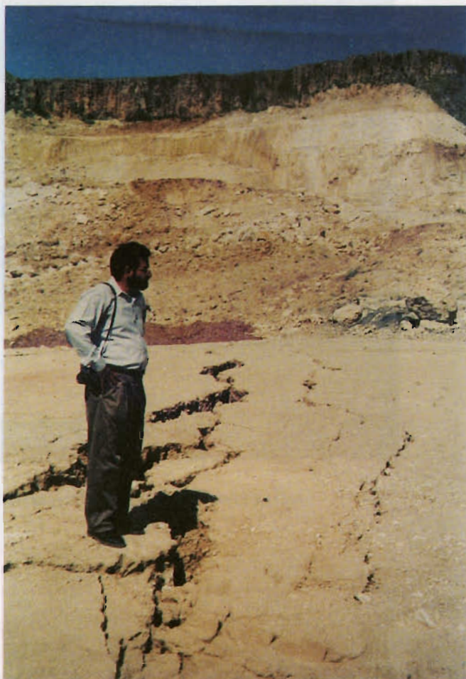
Plate 17: Landslide activity in Aug. 1994 shows slip surface in back-ground and cracks in displaced material along the M1 Motorway Lahore-Islamabad
