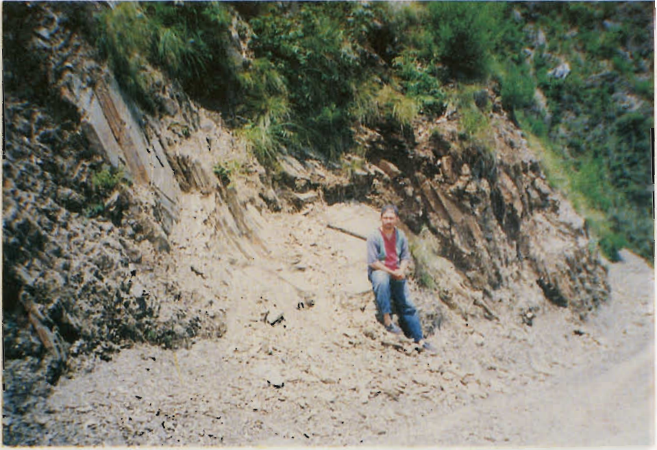
Plate 11: Plane failure in schists at Lower Gali near Muzaffarabad
