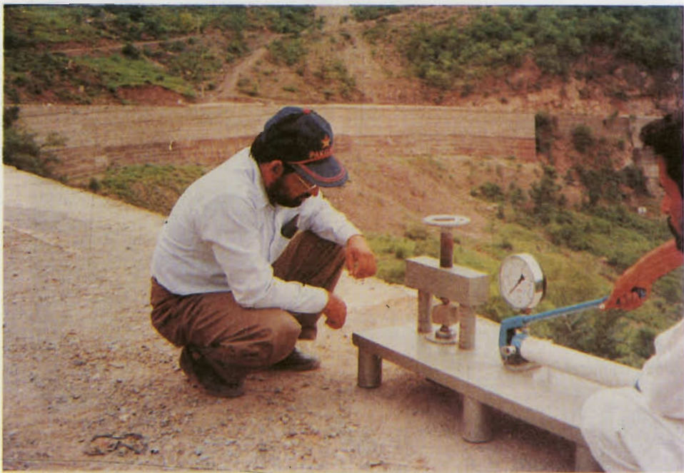
Plate 16: Point load testing of rock at site
