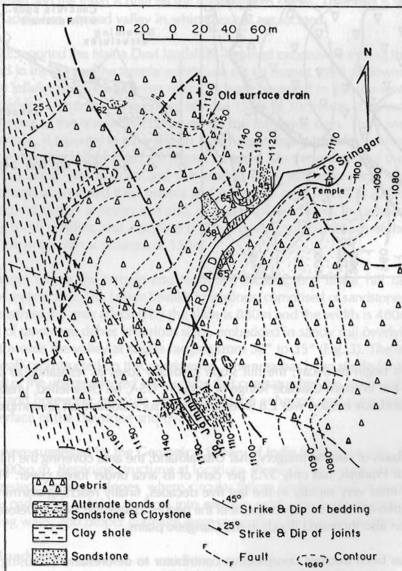
The Central Road Research Institute (CRRI) investigated this slide in June-July 1983, at the request of the Border Road Organisation. The various remedial measures suggested after the investigation include augmentation of surface drainage by constructing a system of catchwater drains, trench drains, chutes, and intercepting drains besides biotechnical stabilisation and installing concrete restraining piles (Fig. 5).
