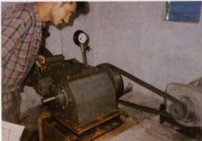
Plate 11: A micro-hydel introduced by the GPIHED is operated by one of the villagers who has received a significant amount of training. The unit is still functioning without any support even after two and a half years.
