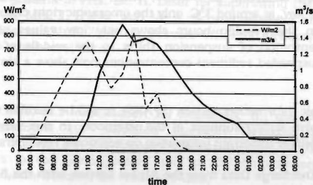
Figure 3: Typical Daily Variation of the Discharge in August Depending upon the Solar Radiation (A time lag between the two elements is clearly to be seen. The discharge starts to increase at 10:00 and decreases continuously from 14:00 to midnight.)
