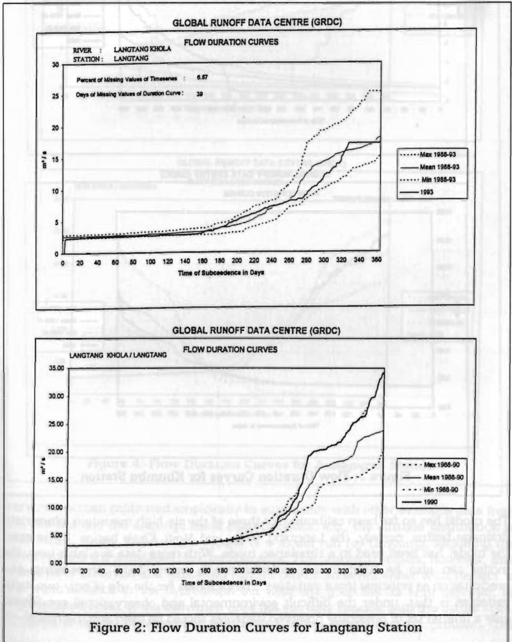
Figure 2: Flow Duration Curves for Langtang Station
