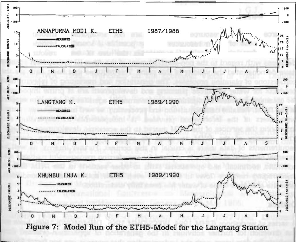
Figure 7: Model Run of the ETH5-Model for the Langtang Station
