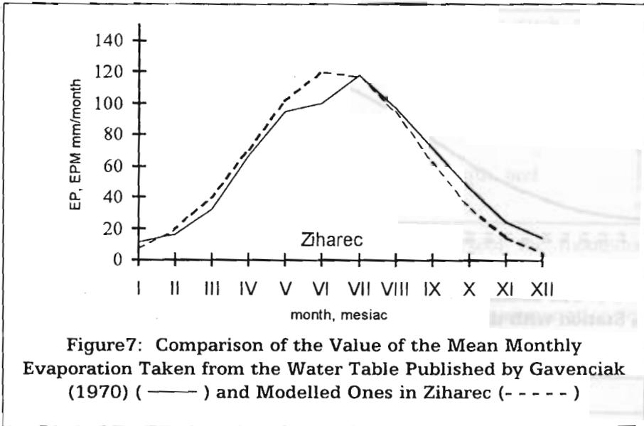
Figure7: Comparison of the Value of the Mean Monthly Evaporation Taken from the Water Table Published by Gavenciak (1970) ( — ) and Modelled Ones in Ziharec ( - - - - )
