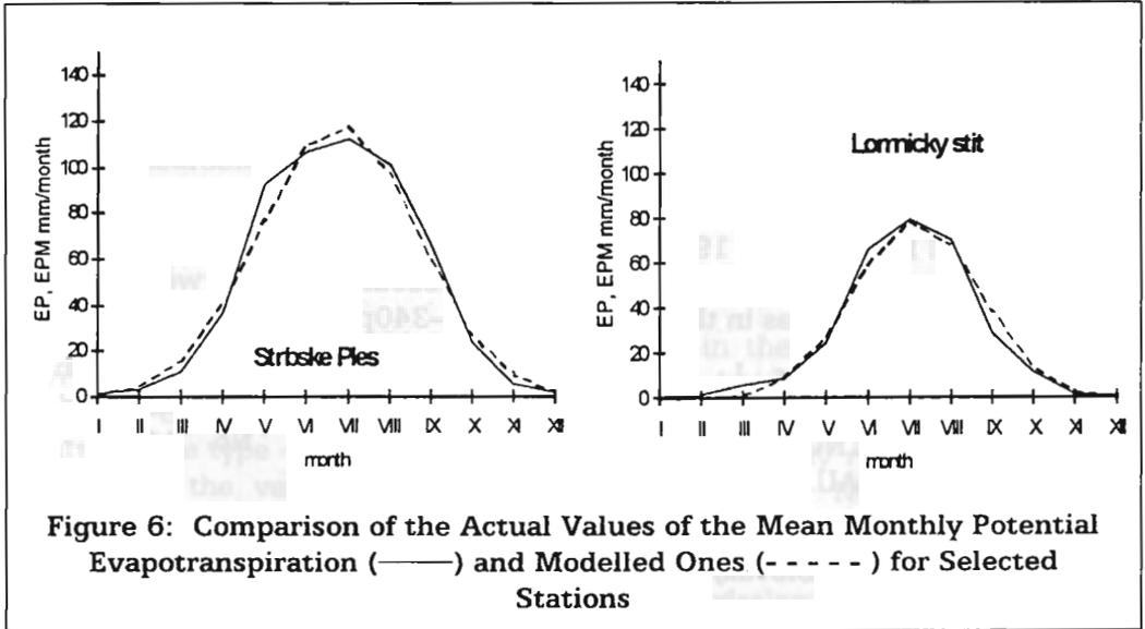
Figure 6: Comparison of the Actual Values of the Mean Monthly Potential Evapotranspiration (—) and Modelled Ones (- - - -) for Selected Stations
