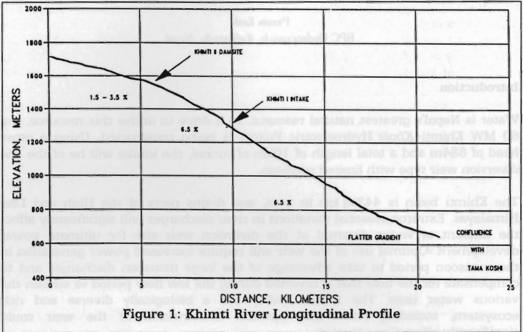
Figure 1: Khimti River Longitudinal Profile
