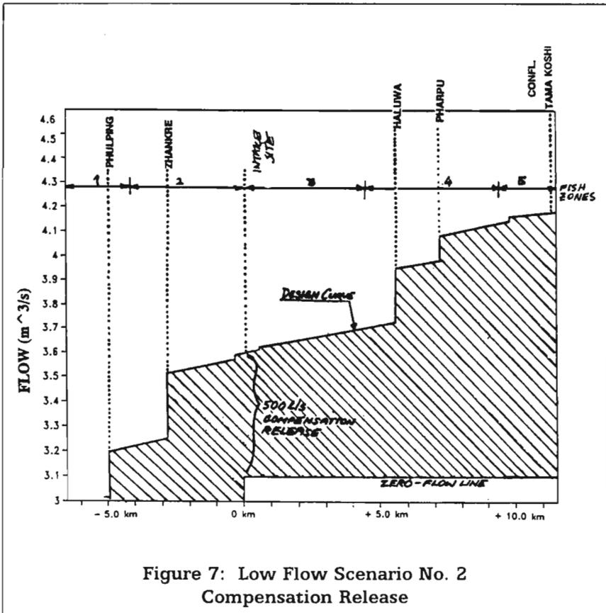
Figure 7: Low Flow Scenario No. 2 Compensation Release
