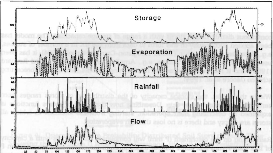
Figure 2: Soil-water Storage, Observed Potential Evaporation (dot-dash line) and Simulated Actual Evaporation (dashed line), Rainfall, and Observed (solid line) and Simulated Flows (dotted line) for the Chinniya *Khola* for the period from March 1992 to October 1993 (Abscissa scale in days, ordinate scales all in mm)
