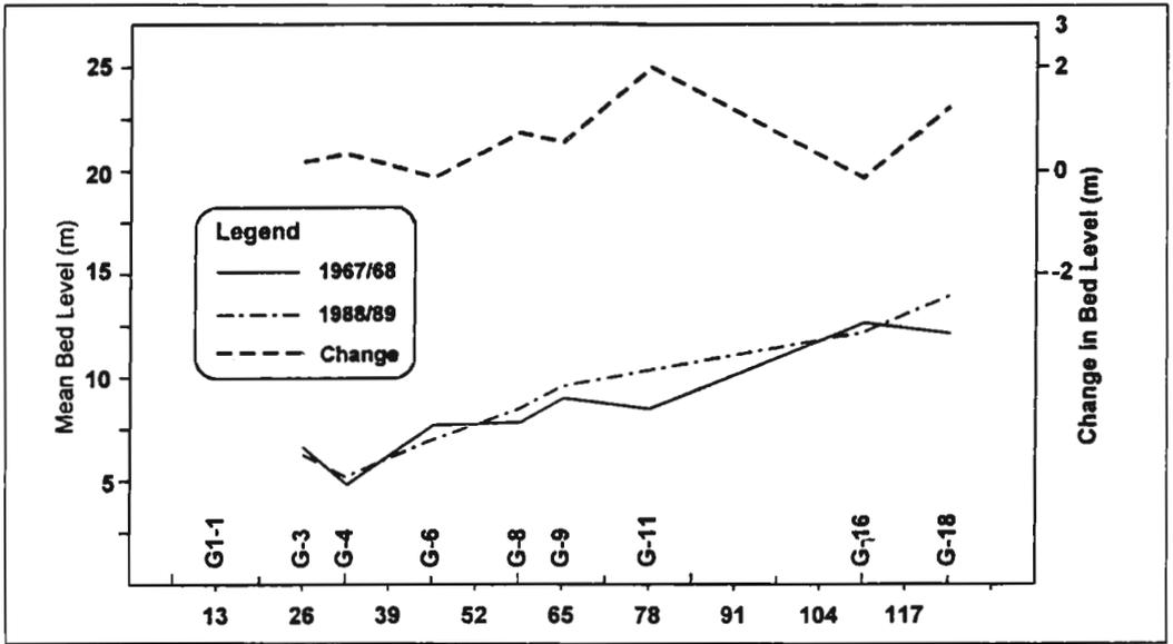
Figure 5: Mean Bed Level for the Lower Ganges
