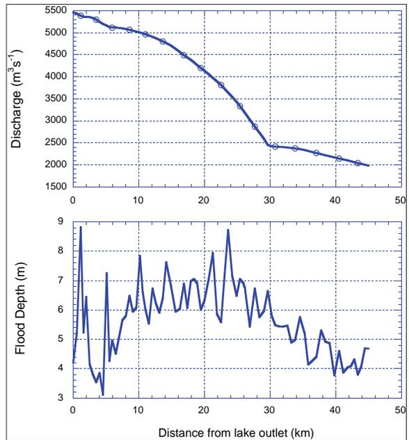
**Figure 4.2:** Estimated peak flow (top) and high flood depth (bottom) in the river
