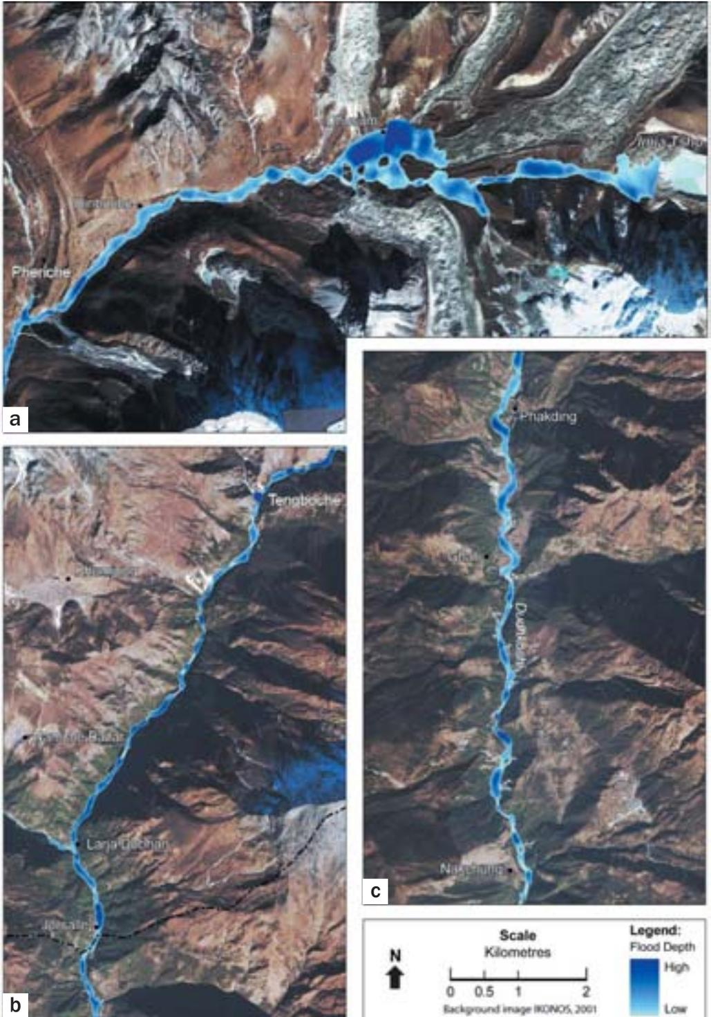
**Figure 4.3:** GLOF hazard in the Imja Khola, Bhoté Koshi, and Dudh Koshi valleys obtained from NWS-BREACH. It depicts stretches between Imja Tsho and Pheriche (a), Tengboche and Jorsalle (b), and Phakding and Nakchung (c)
