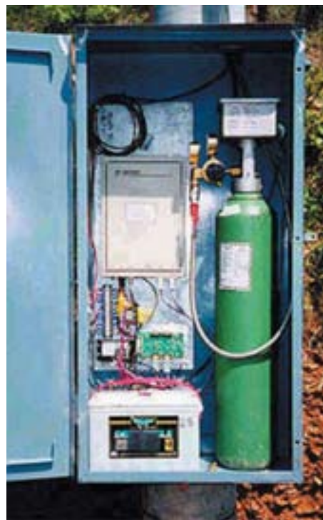
Figure 6.5: An MCC 545 unit with 12 V batteries, air cylinder, and MCC-545A RF modem for relay, mounted inside a lockable shelter
