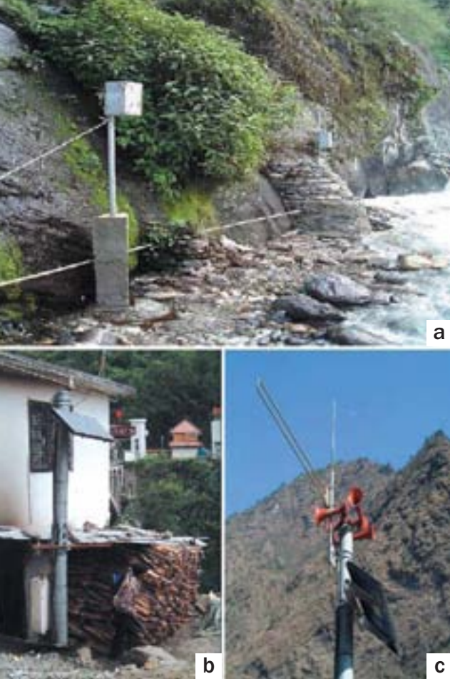
Figure 6.6: GLOF Sensor and early warning system in the Bhote Koshi, (a) Sensor at River Level, (b) Sensor at Friendship Bridge, (c) Early warning system siren
