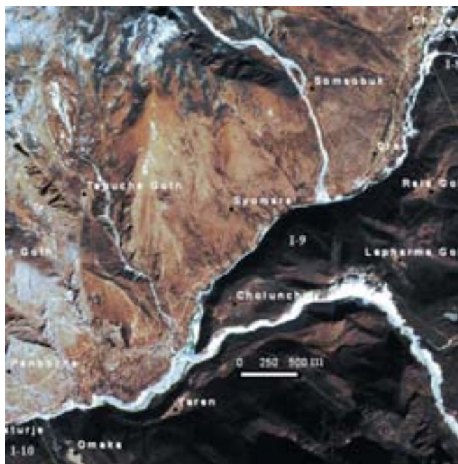
Figure 5.35: Concave bend of the Imja Khola at Syomare where bank scouring is expected in the case of a GLOF
