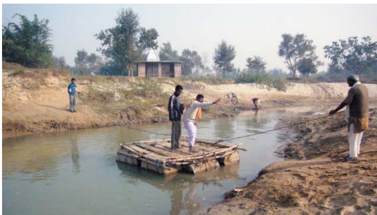
Figure 21: Boat built with local materials (wood, bamboo, and metal containers) to cross the Jamuni River during the flood period. Note a shrine (temple) in the background. (Deuri VDC, Dhanusha District)
