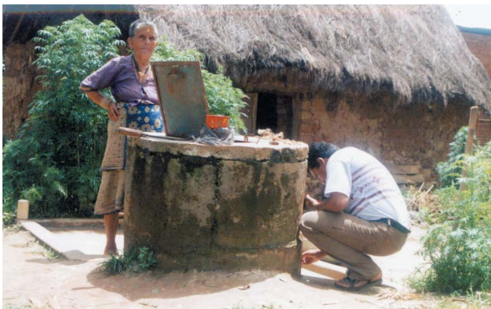
Figure 25: Monitoring the water table in dug wells
