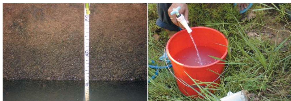
Figure 21: Flow measurement of the spring at Barabot-Dhotra
