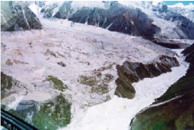
Plate 9.14: Supraglacial lakes being formed in Thorthormi Lake and erosion caused by the 1994 flood on the left lateral moraine.
