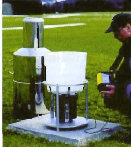
d) PLUVIO 1000 mm with collecting-ring heating device
