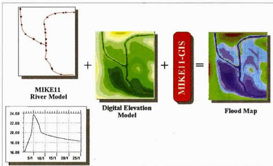
Figure 8: Flood forecasting with numerical modelling and GIS
