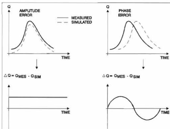
Figure 7: Amplitude and phase errors
