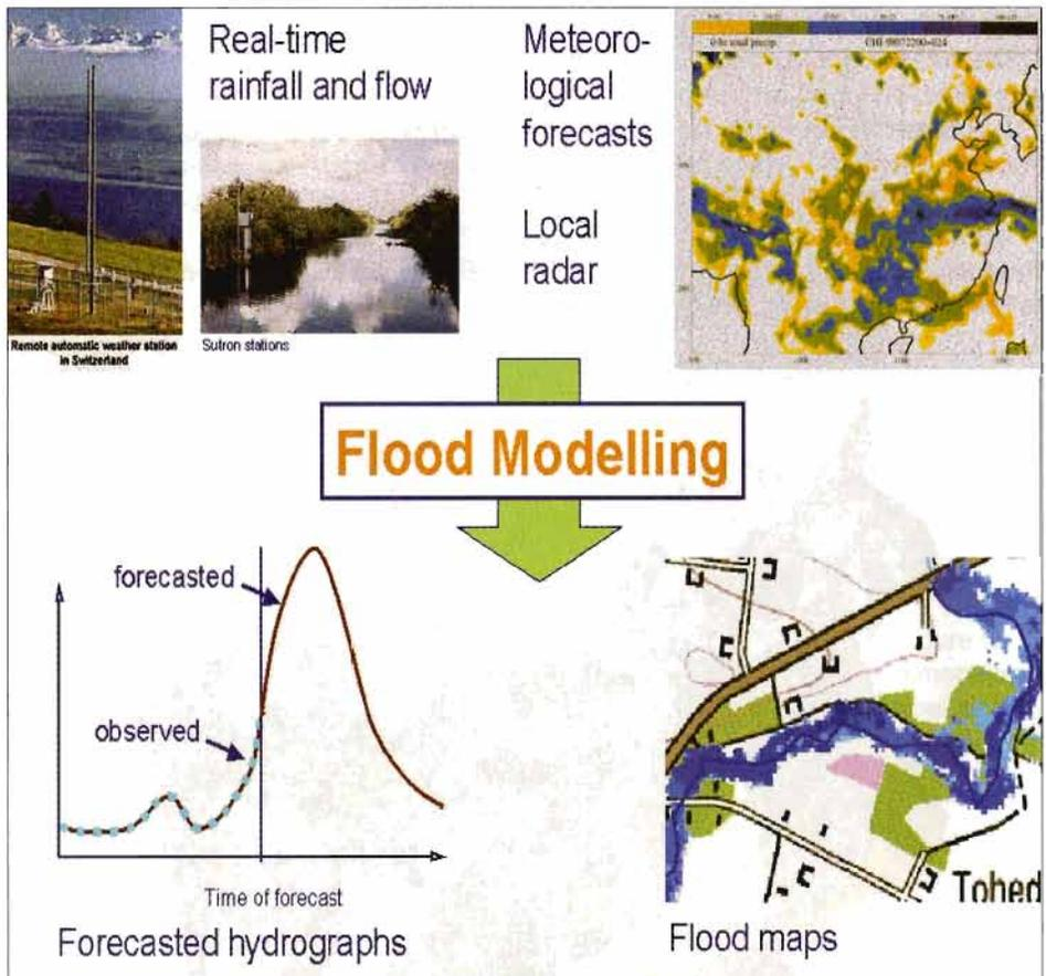
Figure 2: A schematic of a flood forecasting system using models
