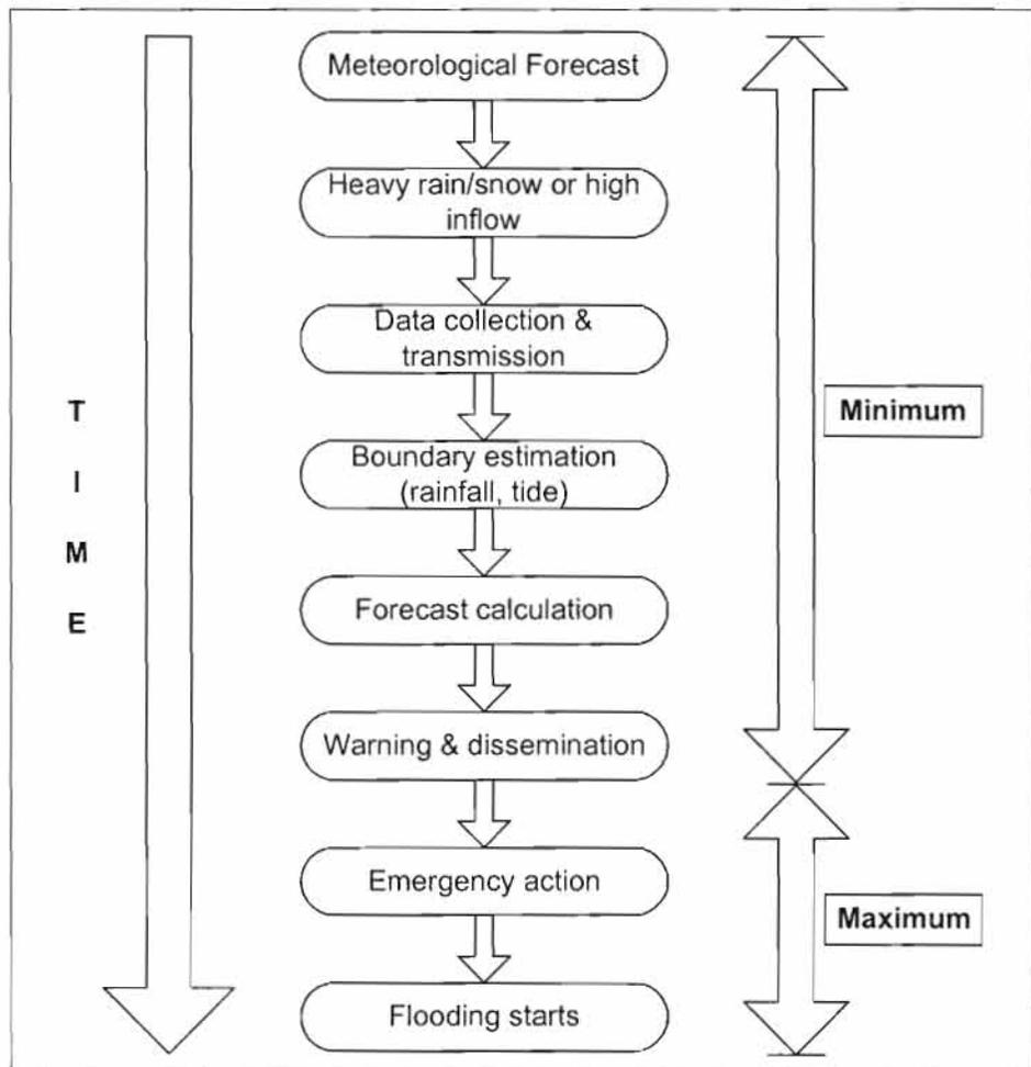
Figure 1: A schematic of the main activities in flood forecasting, warning, and dissemination
