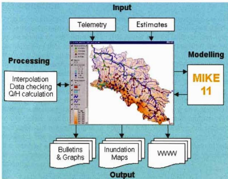
Figure 11: A flood watch system (Source: DHI Water and Environment)
