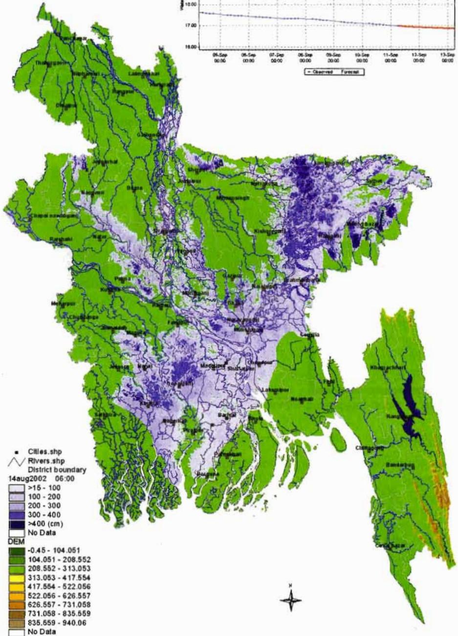
Figure 9: A model generated flood map for the whole of Bangladesh based on flood forecasts from single stations like the one shown in the inset at top
