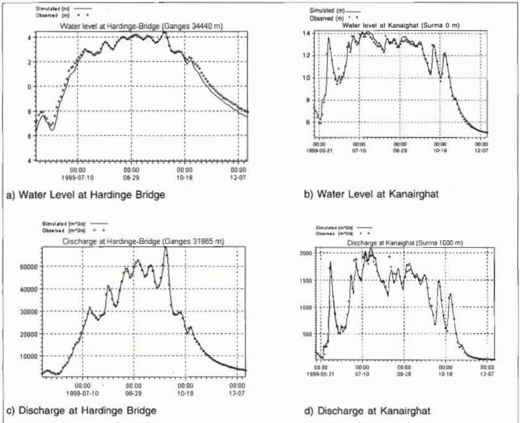
Figure 10: Simulated water levels and discharges (solid line) compared with observed values (dots) at two selected locations in the river system.
