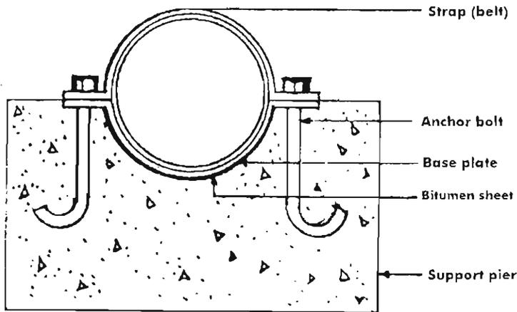
**Figure 5.10: Cross Section through a Support Pier**
