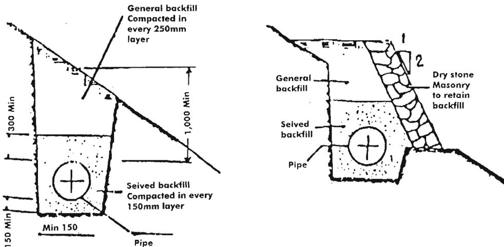
**Figure 5.9: Section Through Pipe Buried in Different Ways**
