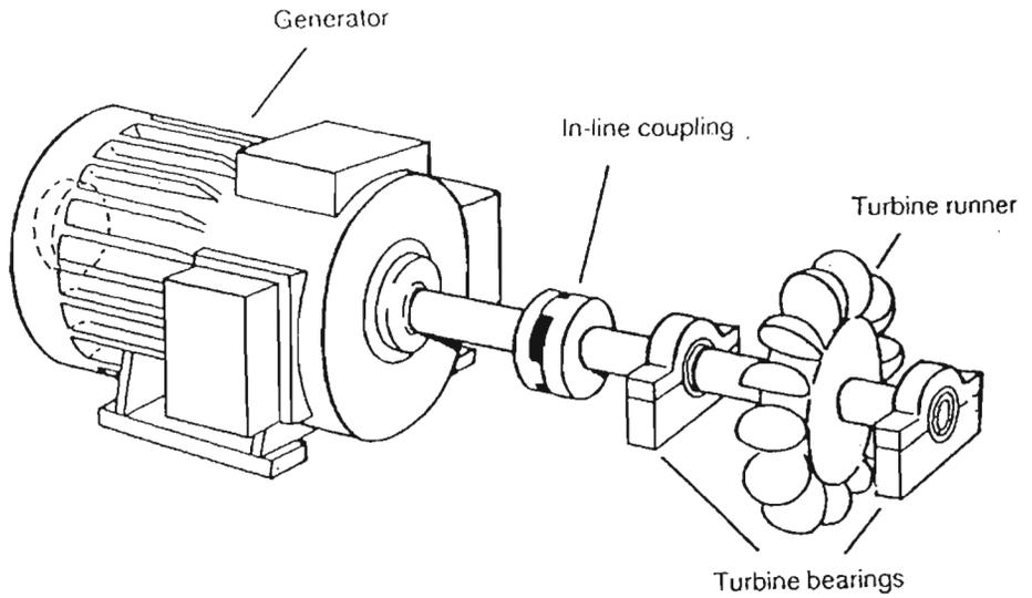
**Figure 5.1: Direct Drive Turbine and Generator System**
