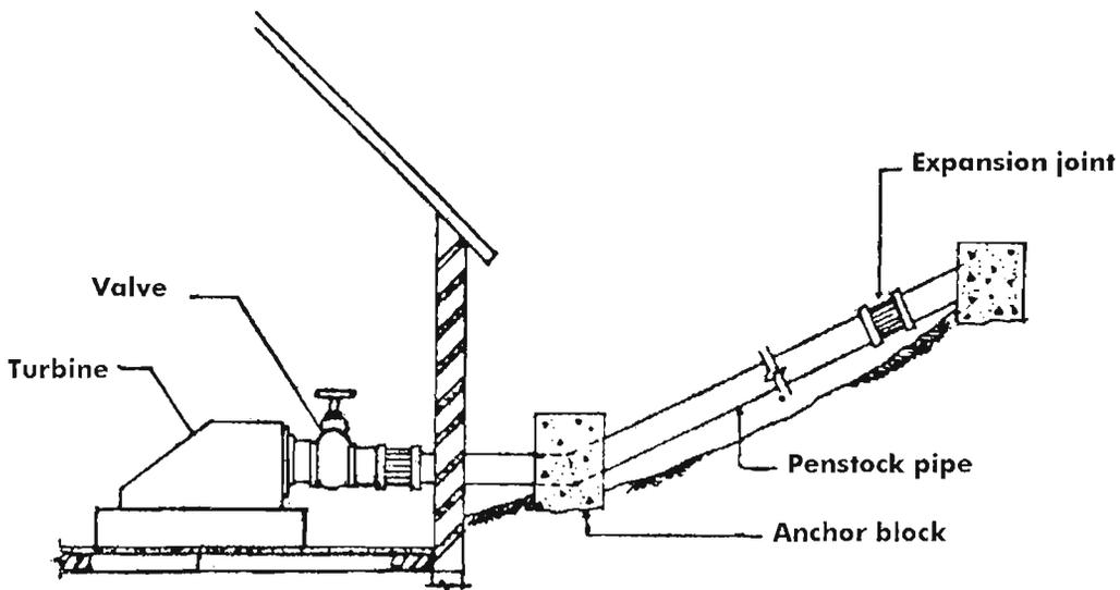
**Figure 5.6: Cross-section through a Powerhouse and Anchor Block**
