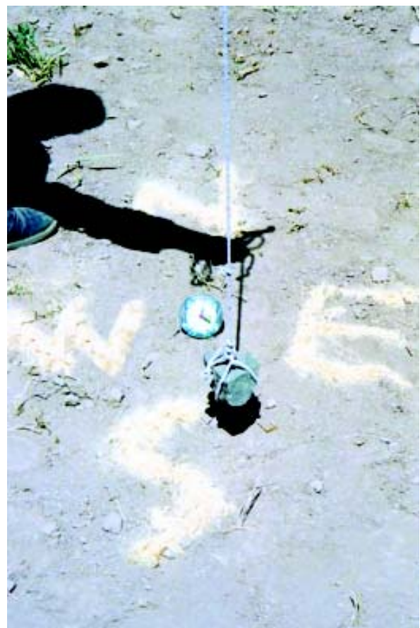
Figure 27: Finding south with a plumb line
