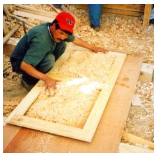
Figure 45: Assembling the door
