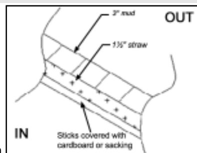
Figure 60: Roof composition
