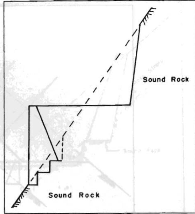
Figure 11. A Cement masonry wall can be constructed economically in rocky areas because benching of the foundation is possible and the backfill wedge may also be smaller.
