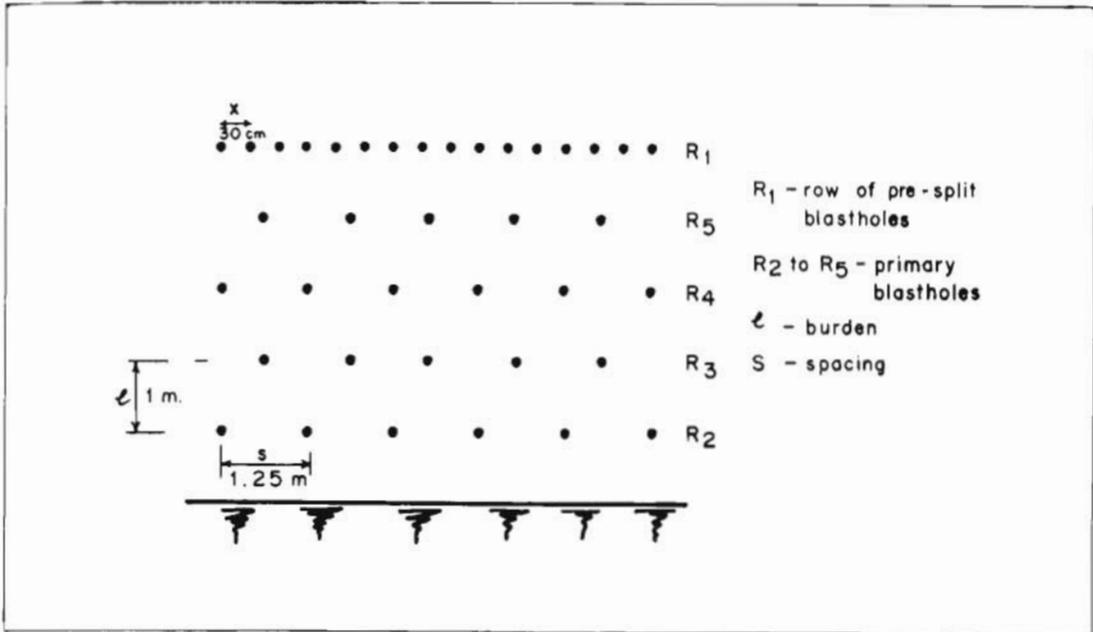
**Figure 16b. Plan view of 16a: a staggered pattern of blasting**
