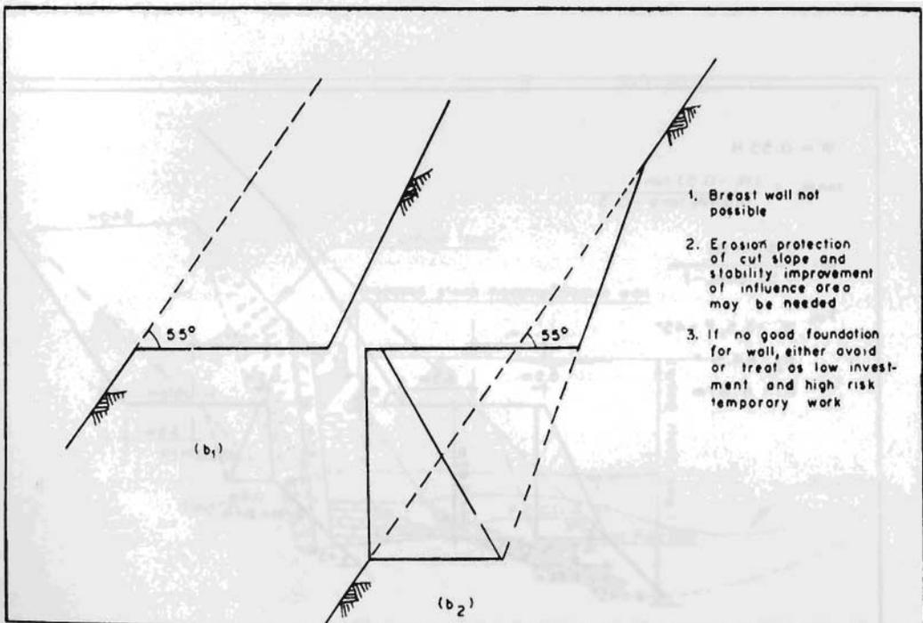
**Figure 9.** On very steep slopes, breast wall construction is not feasible. By shifting the centre line horizontally and providing a back-battered retaining wall towards the downhill side of the road, the volume of excavation is reduced.
