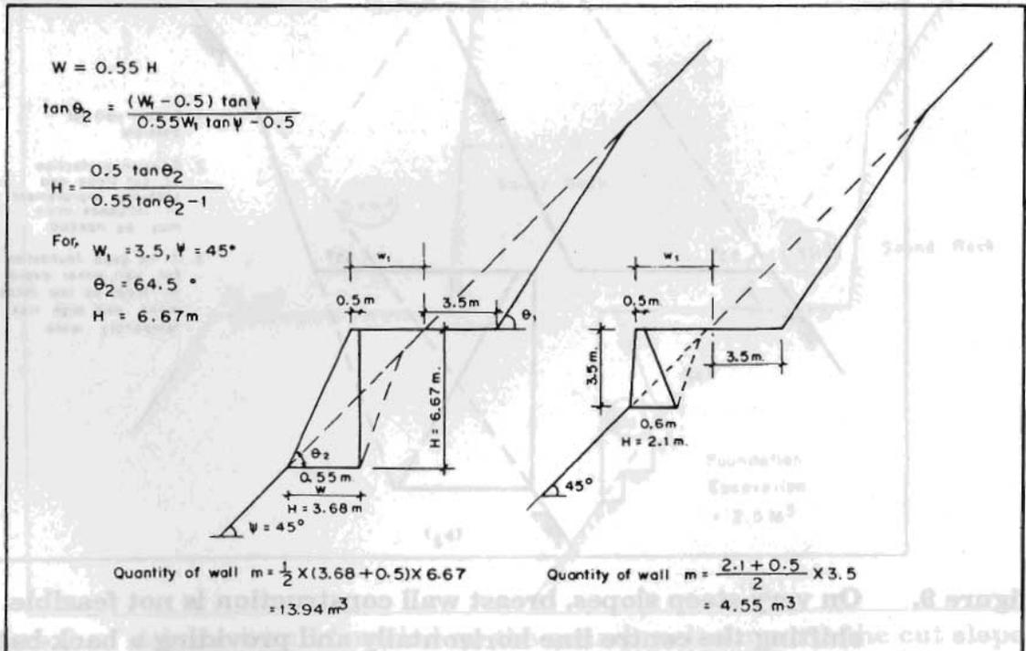
Figure 12. A Back-battered, Front-battered Retaining Wall
