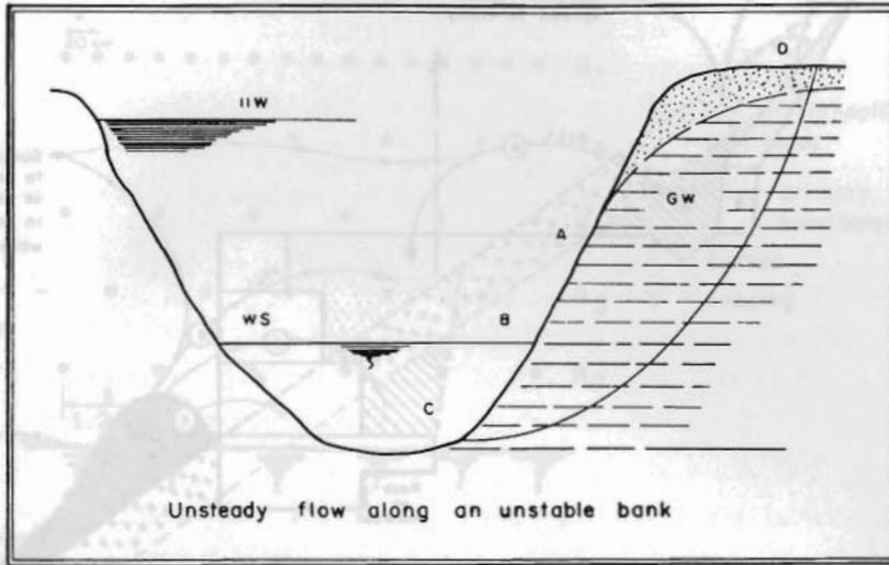
Figure 13. A high water table in the bank slope, due to change in flood level, weakens the bank
