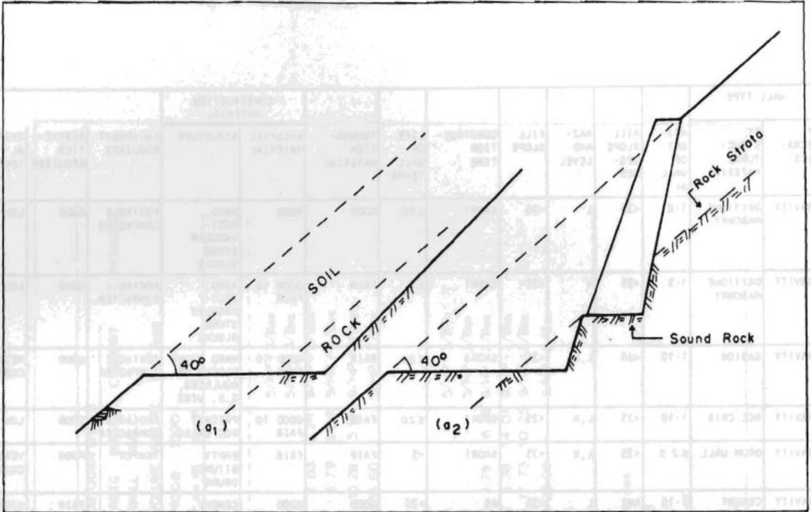
**Figure 6.** In rocky areas, where excavation is difficult and expensive, the centre line shifts towards the valley and reduces the height of cut and volume of excavation to a great extent.
