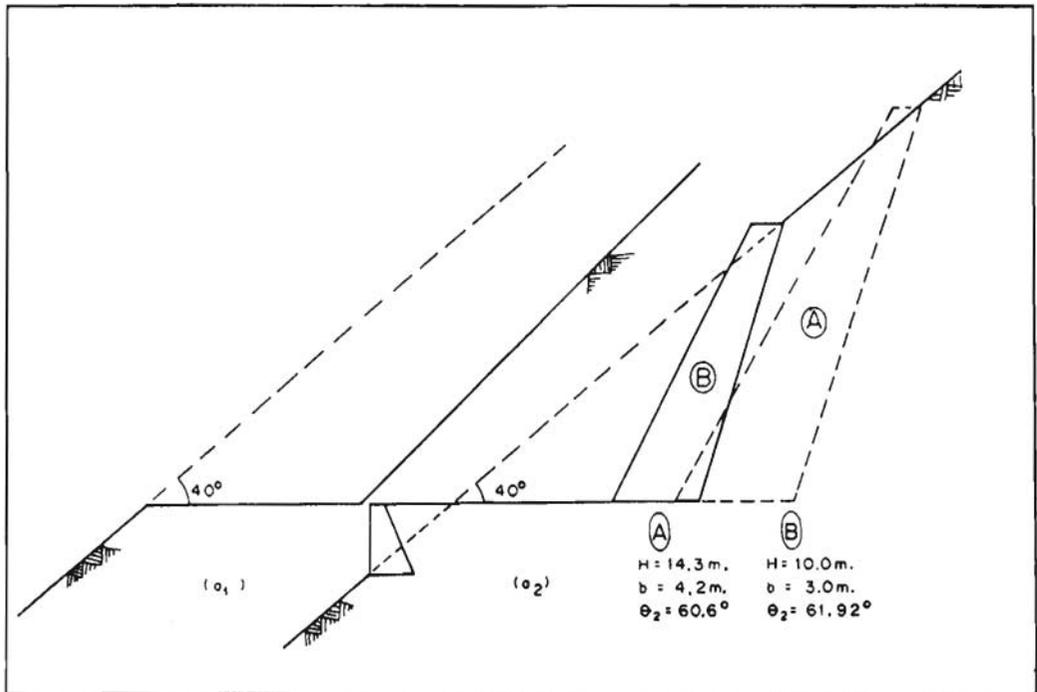
**Figure 8.** Minimising height of cut on steep slopes is possible by providing breast walls and shifting the centre line horizontally as shown in the figure to the right.
