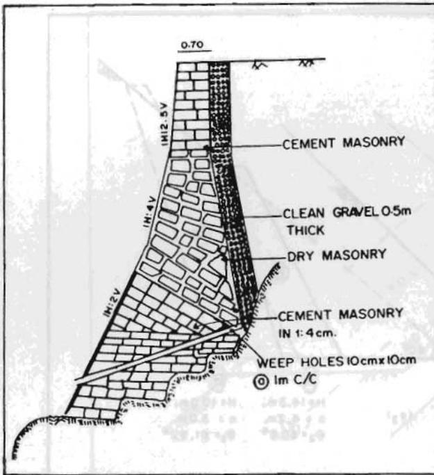
Figure 10. A Composite wall (consisting of dry masonry and cement masonry) is suitable and economical whenever the foundation is sound.
