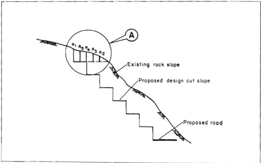
Figure 16a. An illustrative diagram for pre-split blasting
