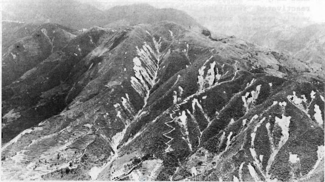
Photo III Near Lele, Lalitpur District. After a prolonged rainfall in Sept. 1981, this slope failed en masse in spite of thick shrub cover. Such catastrophic events are common on certain landforms within the Nepal Himalayas but are difficult to predict.
