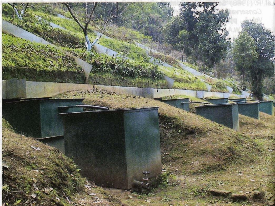
View of the lower portion of one of the soil erosion plots showing the collecting tanks for the runoff from four of the different treatment strips, as described in the next chapter.
