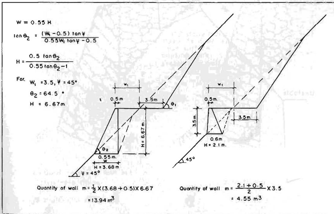
Fig. 24.31 Back-battered versus front-battered retaining wall
