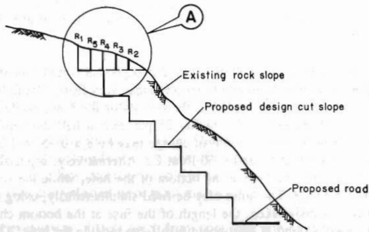
Fig. 24.56 Illustrative diagram for pre-split blasting
