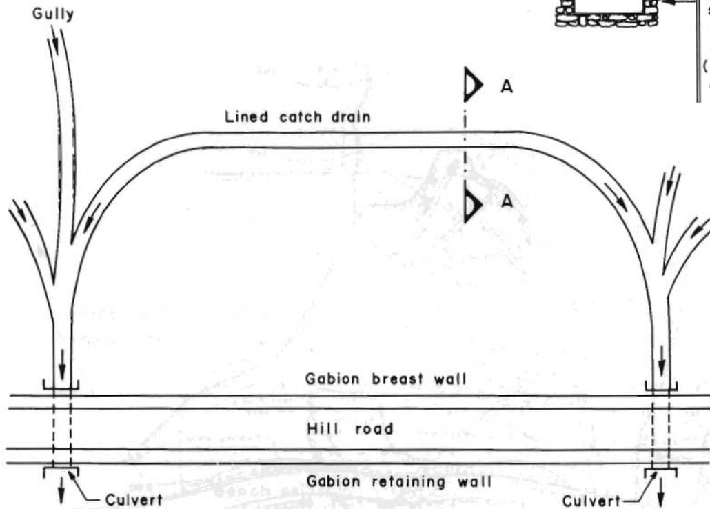
Fig. 24.72 Surface drainage system for hill slopes with unstable talus deposit
