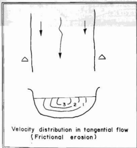
Fig. 24.83 Velocity distribution in tangential flow (frictional erosion)
