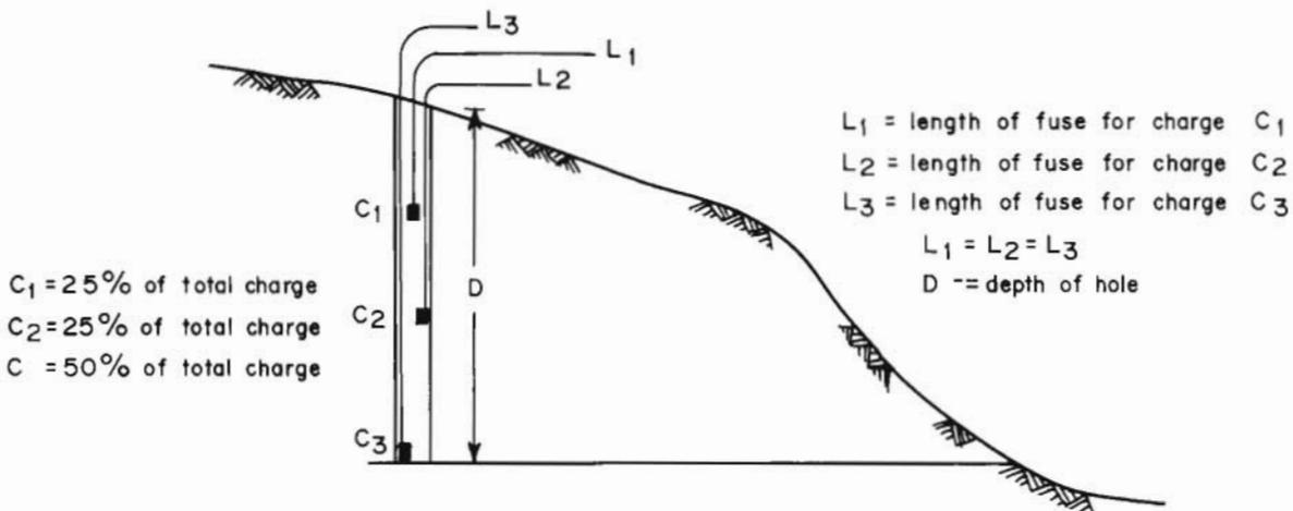
Fig. 24.58 Details of charge placement of pre-split holes of row R
