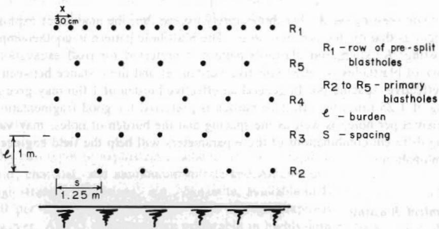
Fig. 24.57 Plan view of A - staggered pattern of blasting
