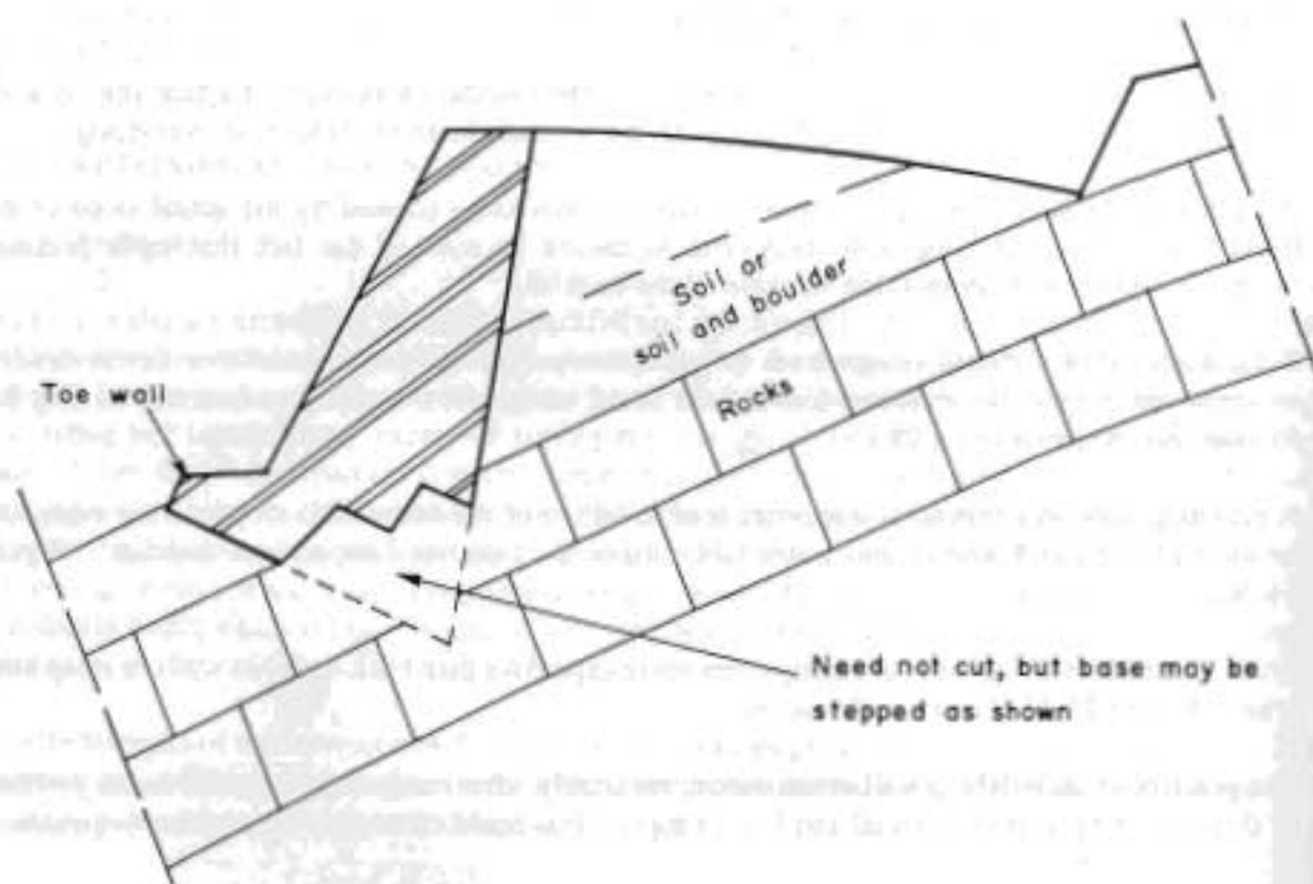
Fig. 24.29 Avoiding unnecessary cut for retaining wall on rock
