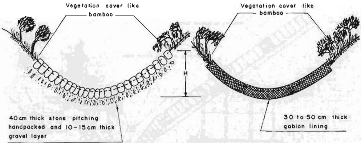
Fig. 24.24 Gully bed lining for gully control
