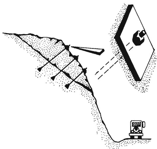
b) Tensioned anchors installed
