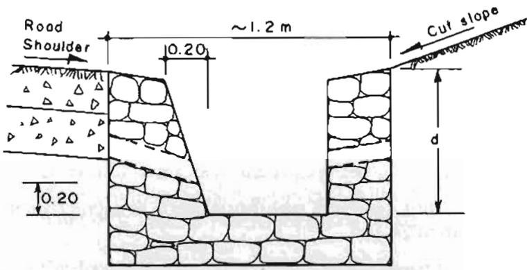
(a) Rectangular drain to withstand traffic surcharge adjacent to drain
