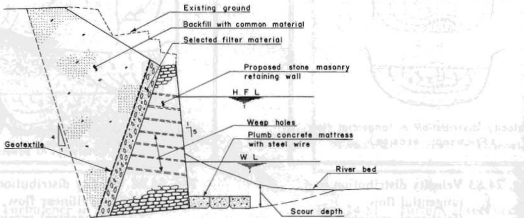
Figure 24.87 River training work with type 'B' launching apron
