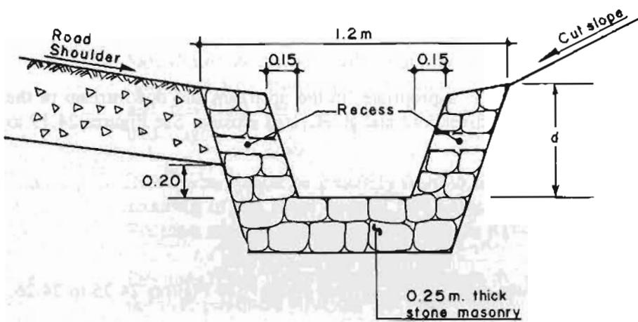
(b) Trapezoidal stone masonry drain (for no traffic surcharge load condition)
