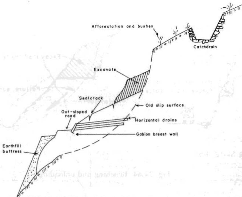
Fig. 24.66 Stabilization of old landslide area
