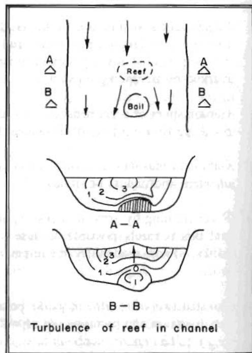
Fig. 24.81 Turbulence at reef in channel (Kolk erosion)
