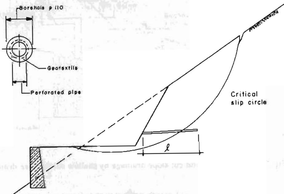
Fig. 24.27 Horizontal drains
