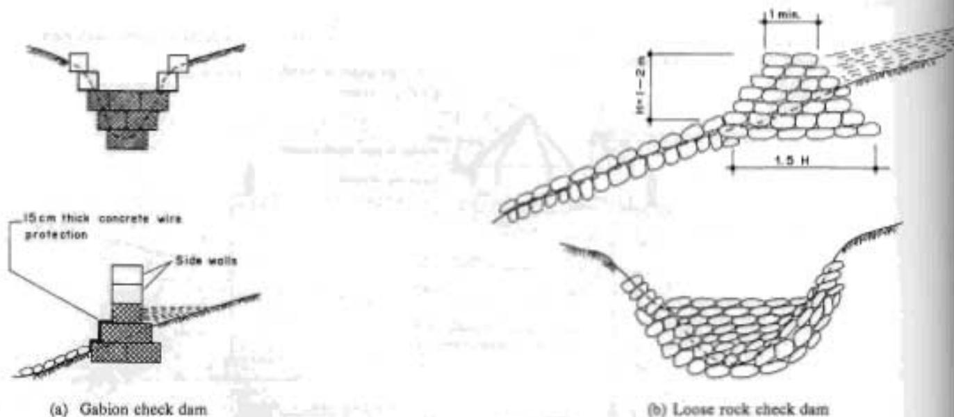
Fig. 24.19 Check dams for gully control
