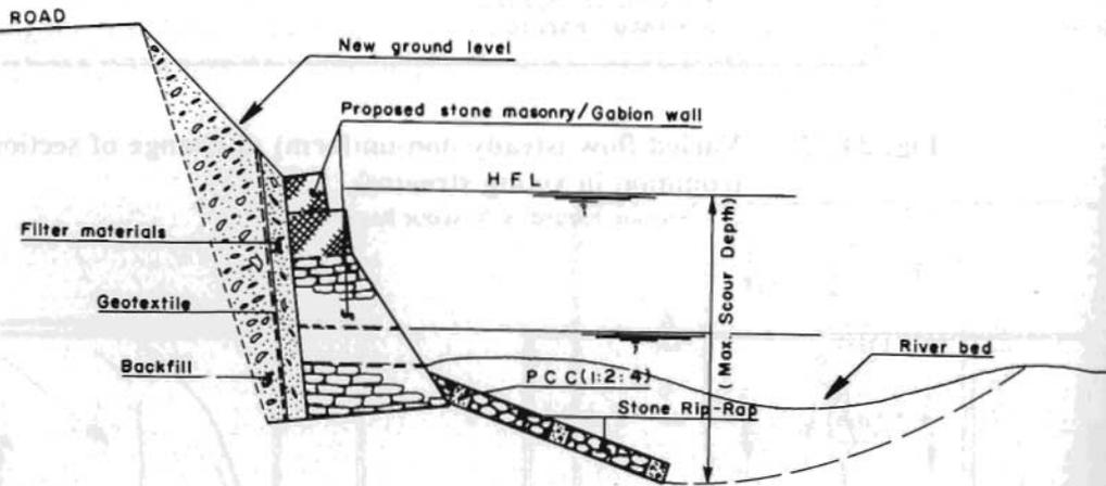
Figure 24.86 Revetment for river training with type 'A' launching apron
