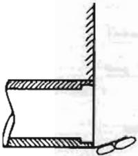
c) Endgrooved culvert pipe
