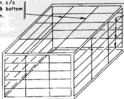
Provide 6mm  $\phi$  20cm c/c All around 4 faces in horizontal direction & 6mm  $\phi$  50cm. c/c vertically.
