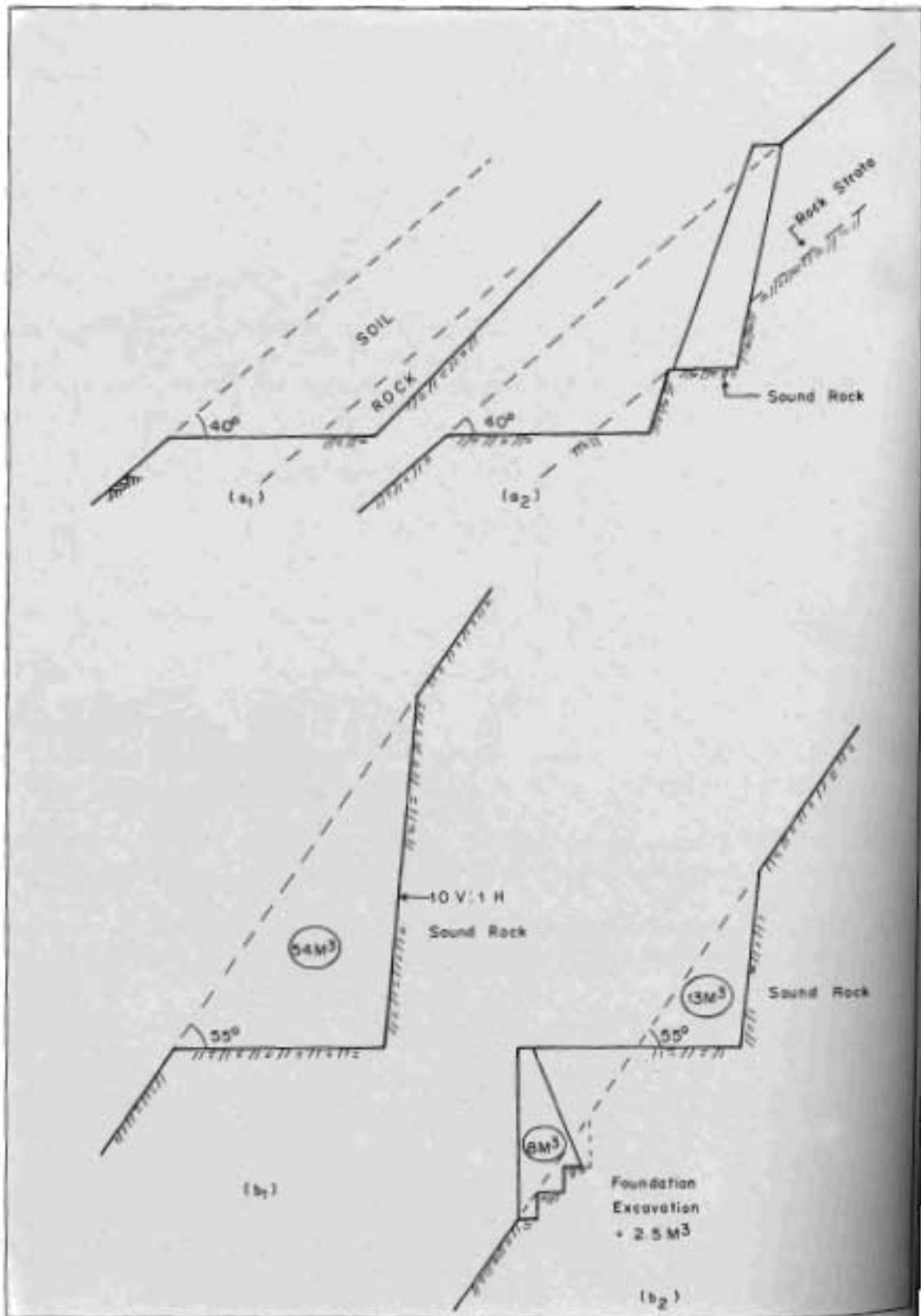
Fig. 24.2 Minimizing height of cut in rock and soil areas and rocky areas
