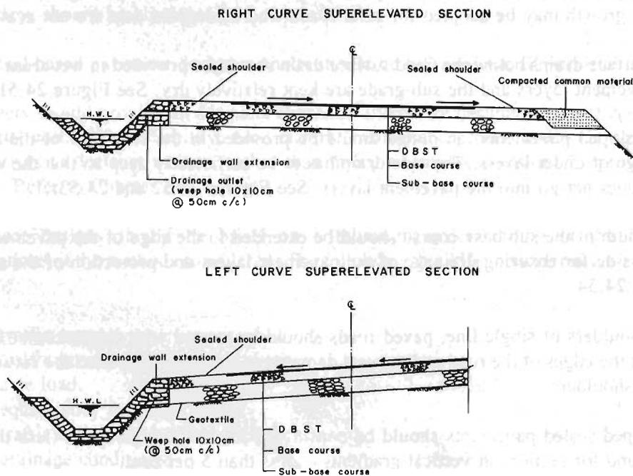
Fig. 24.52 Typical pavement section
