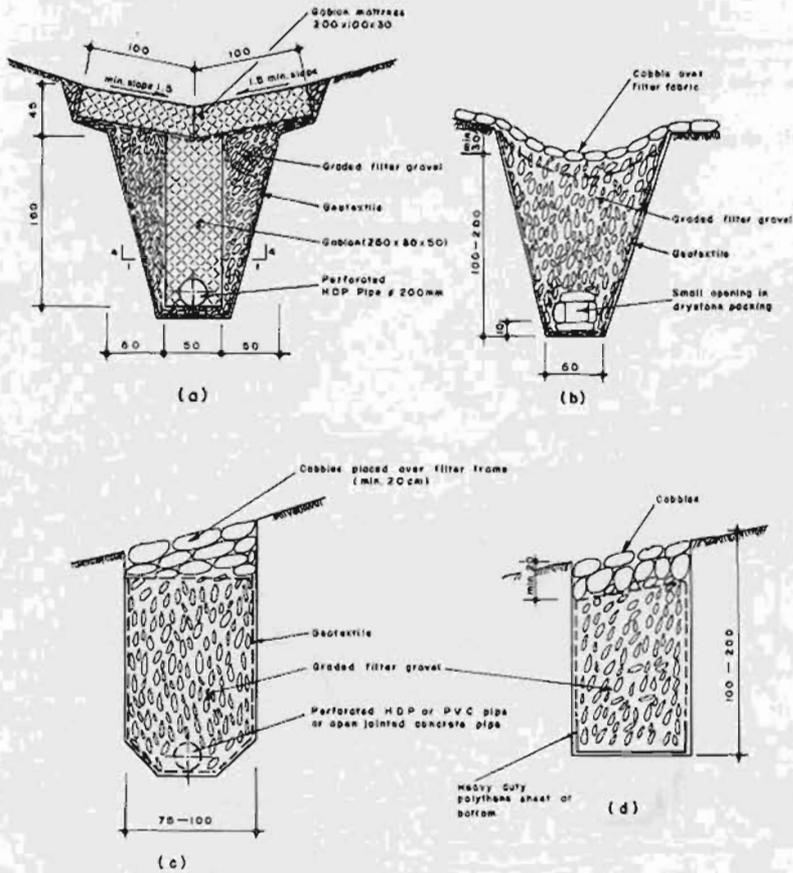
Fig. 24.25 Landslide and cut slope drainage by shallow sub-surface drains
