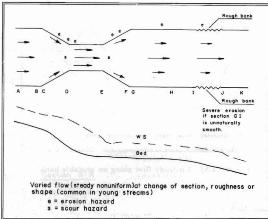
Fig. 24.82 Varied flow (steady non-uniform) at change of section, roughness or shape (common in young streams)
