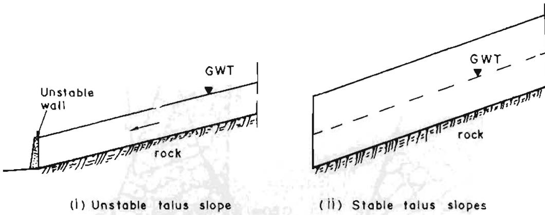
Fig. 24.30 Thin cover of talus/debris is likely to fail even on gentle slopes
