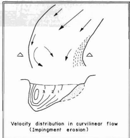
Fig. 24.84 Velocity distribution in curvilinear flow (impingement erosion)
