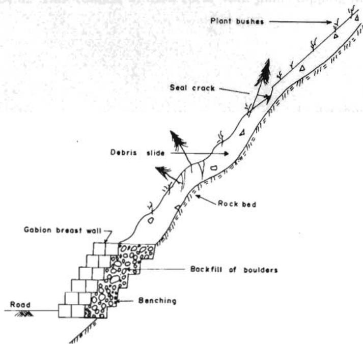
Fig. 24.67 Stabilization of minor landslides by gabion breast walls
