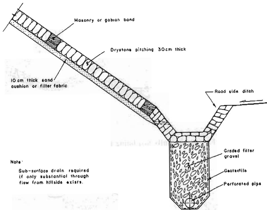
Fig. 24.26 Saturated slope drainage
