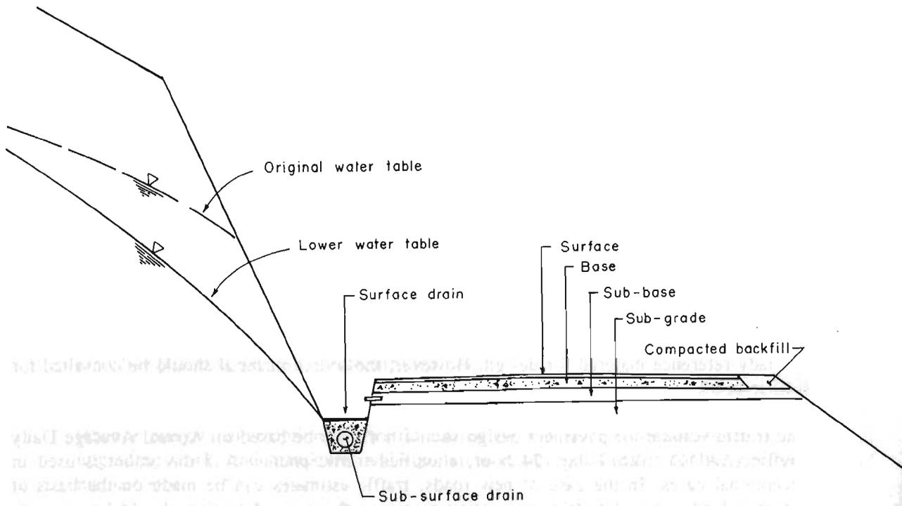
Fig. 24.51 Sub-surface drain to protect pavement in wet areas in soils
