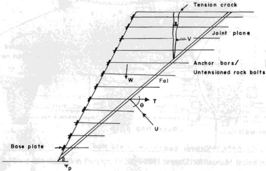
Fig. 24.69 Reinforcement of rock cut with anchor bars
