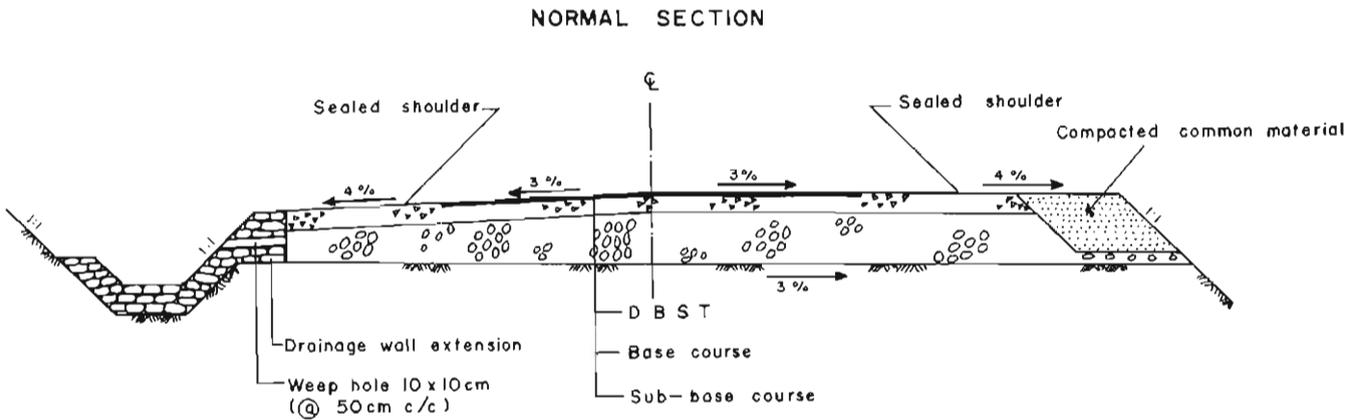
Fig. 24.53 Typical pavement section, normal section
