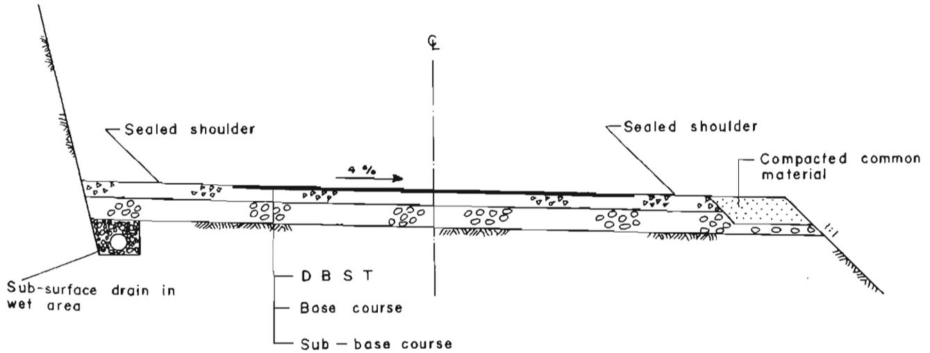
Fig. 24.54 Typical outsloped pavement section
