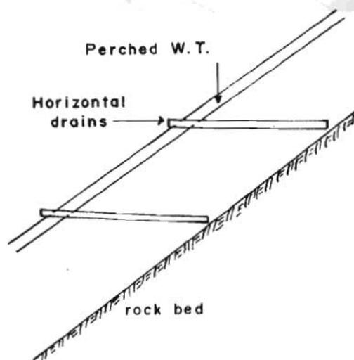
Fig. 24.73 Surface drainage system for stabilization of unstable talus debris
