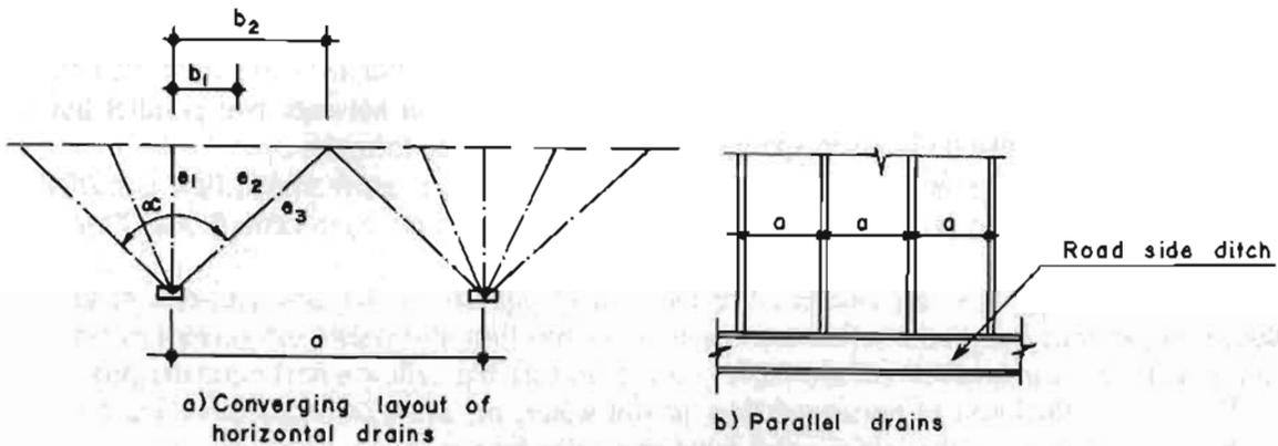
(a) Converging layout of horizontal drains
