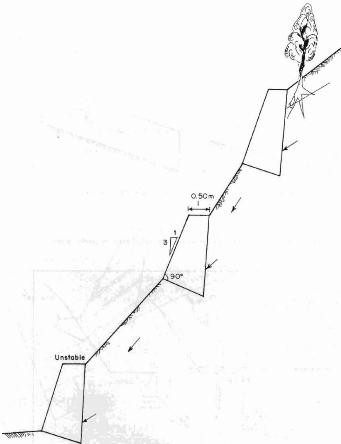
Fig. 24.32 Destabilization of slope by series of retaining walls
